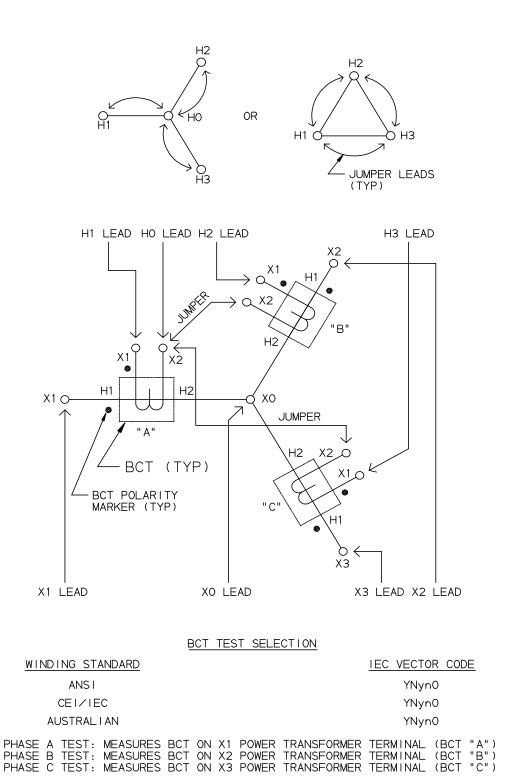
Figure 4-9. Setup for Testing BCT Mounted on Wye Winding of a Three-Phase Transformer
