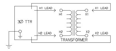
Figure 4-1. Setup for Testing Single-Phase Transformer
