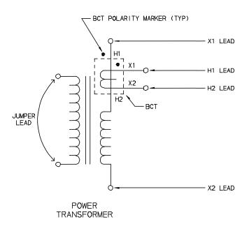
Figure 4-7. Setup for Testing BCT Mounted on Single-Phase Two-Winding Transformer
