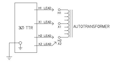
Figure 4-2. Setup for Testing Single-Phase Autotransformer
