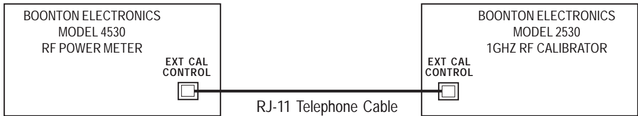
Figure 3-20. External Calibrator Connection
