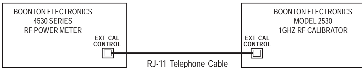
External Calibrator Connection Diagram
