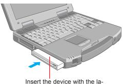
Insert the device with the label side facing up.
