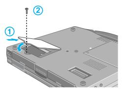
4 Put the cover back into place, then fasten the screw
