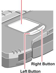
Use the touch pad to move the cursor on the display and perform normal computer operations.
