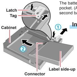
The battery pack can be used as a second battery by installing into the multimedia pocket. (An optional second battery pack adaptor (CF-VAB721) is required to use the second battery).
