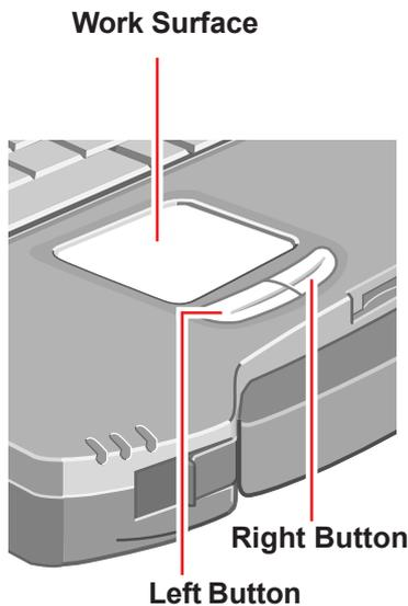
Use the touch pad to move the cursor on the display and perform normal computer operations.
