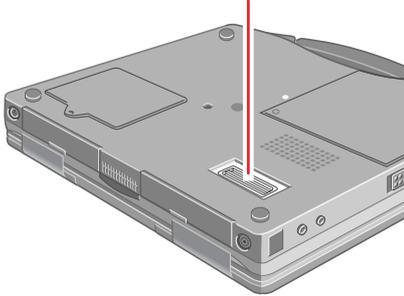
A port replicator is available as an option (CF-VEB481). This device eliminates the hassles of having you connect/disconnect the various cables when carrying your computer around and allows a variety of peripherals to be connected including a headphone or microphone, etc.
