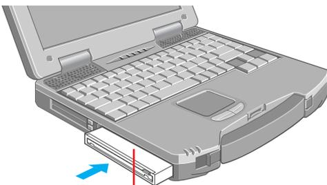
Insert the device with the label side facing up.
