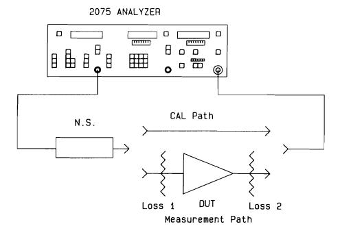
Figure 3-28. LOSS COMPENSATION
