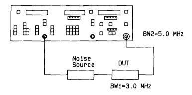
Figure 3-24. BANDWIDTH COMPENSATION - EXAMPLE 1
