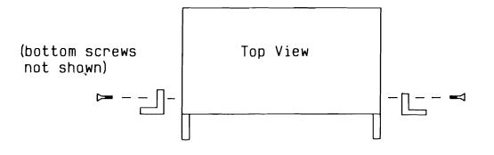
Figure 2-3. INSTALLATION OF RACK MOUNTS
