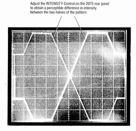
Figure 3-30. TEST PATTERN 2 OSCILLOSCOPE DISPLAY
