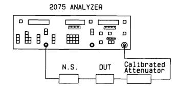
Figure 3-16. MANUAL Y-FACTOR MEASUREMENT
