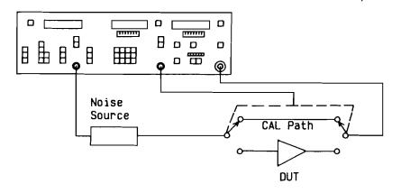
Figure 3-19. SETUP WITH EXTERNAL RELAYS USED TO AUTOMATE CALIBRATION
