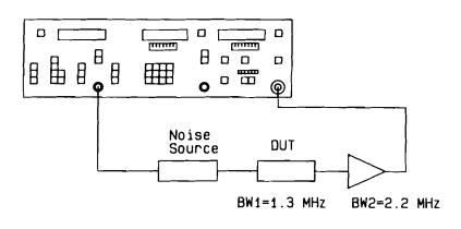
Figure 3-25. BANDWIDTH COMPENSATION - EXAMPLE 2
