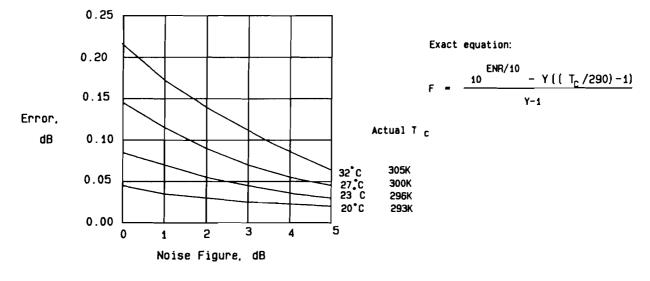
Figure 3-29. ERROR CAUSED BY T<sub>COLD</sub> DEVIATION FROM 290 K
