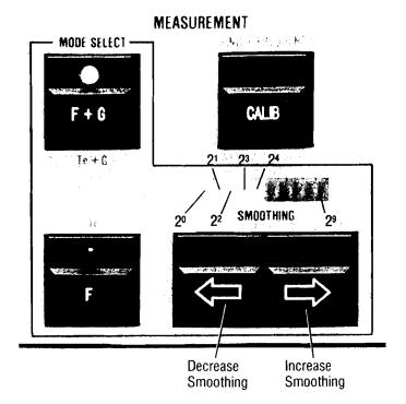
Each light bar, when illuminated, indicates a power of 2 increase in the number of readings taken before the result is displayed.
