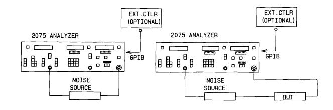
Figure 3-5a. TEST CONFIGURATION 1 Calibration
