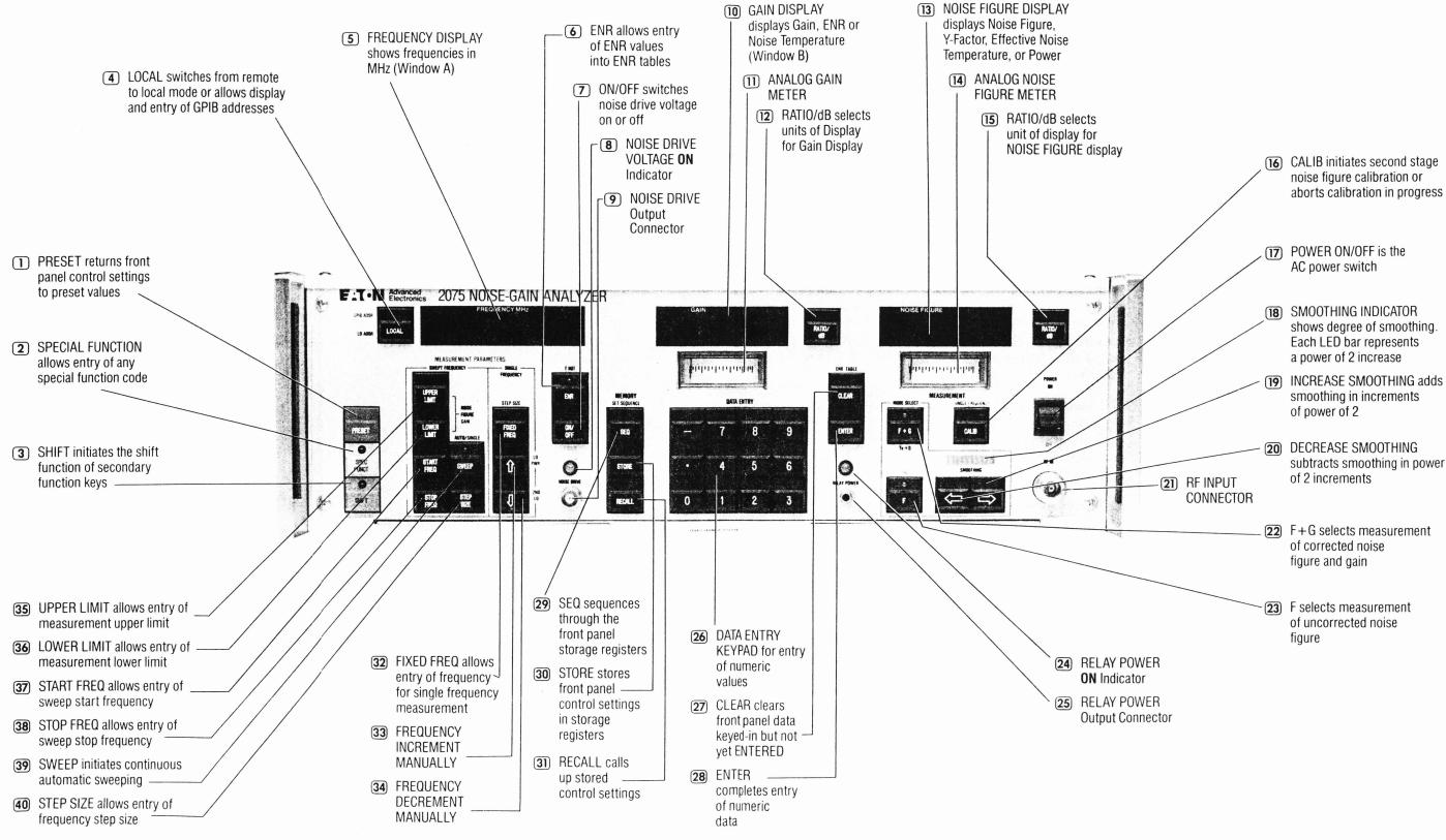
Figure 3-1. 2075 FRONT PANEL CONTROLS AND INDICATORS
