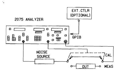
Figure 3-6. EXTERNAL RELAYS AUTOMATE CALIBRATION AND MEASUREMENT PATHS
