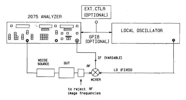
Figure 3-9b. TEST CONFIGURATION 3 MEASUREMENT
