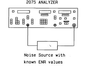
Figure 3-15a. ENR SETUP - CALIBRATION
