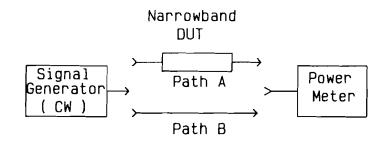
INSERTION LOSS MEASUREMENT WITH POWER METER Figure 3-26.
