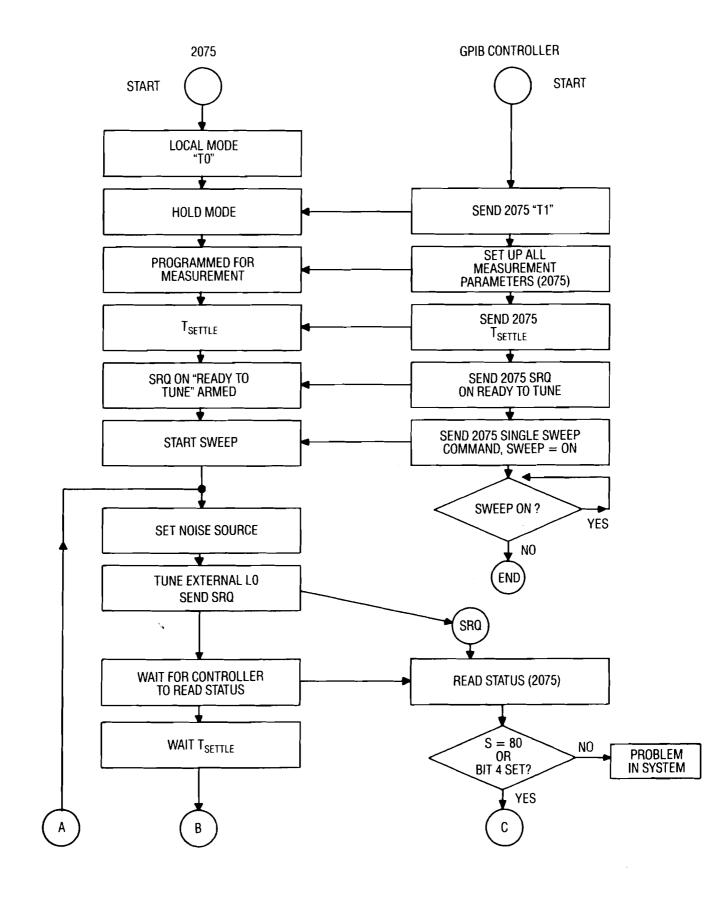
Figure 4-8. FLOWCHART FOR SRQ ON READY TO TUNE
