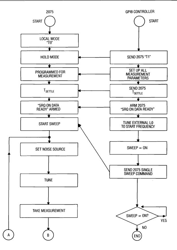
Figure 4-9. FLOWCHART FOR SRQ ON DATA READY
