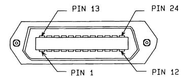
Figure 2-5. GPIB CONNECTOR
