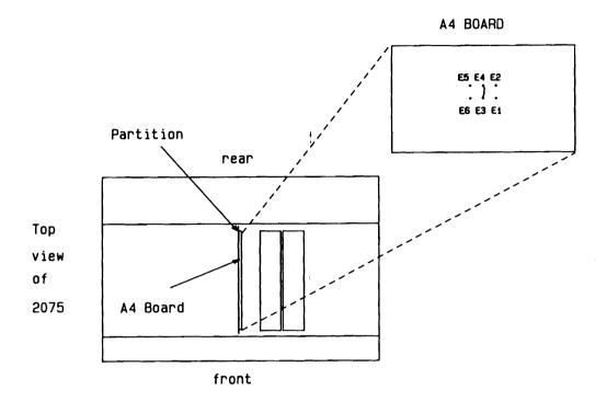
Figure 2-2. EXTERNAL RELAY VOLTAGE SELECTION
