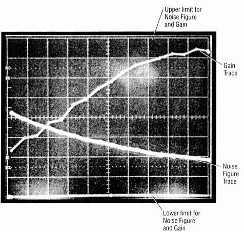
Figure 3-31. NOISE FIGURE AND GAIN OSCILLOSCOPE DISPLAY
