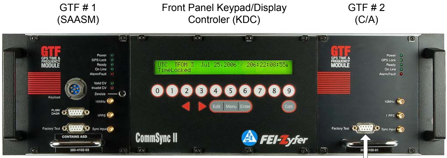
Figure 4-1 CommSync II Front View - GTF
