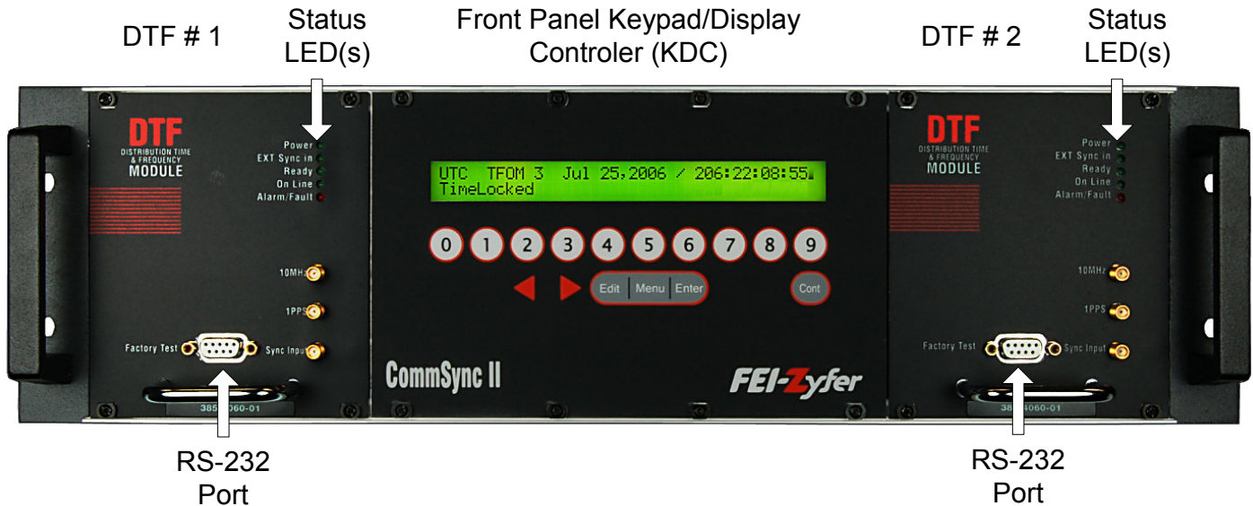
Figure 6-4 Commsync II Front Panel Port and Indicator Locations – DTF Systems
