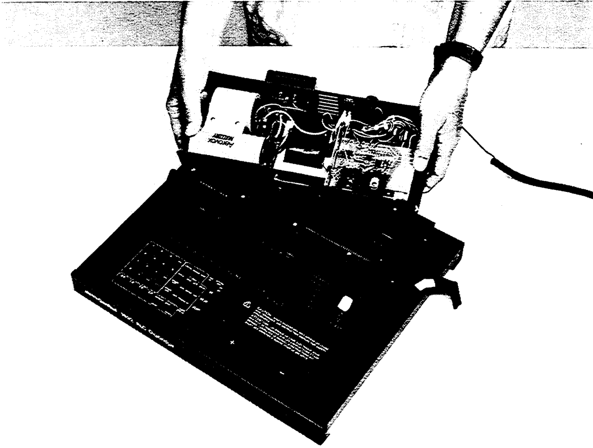
Figure 5-6. Removal of the power supply from the 1692 Digibridge. The ribbon cable must be disconnected first. The display board can be removed first or left in place, as shown here.
