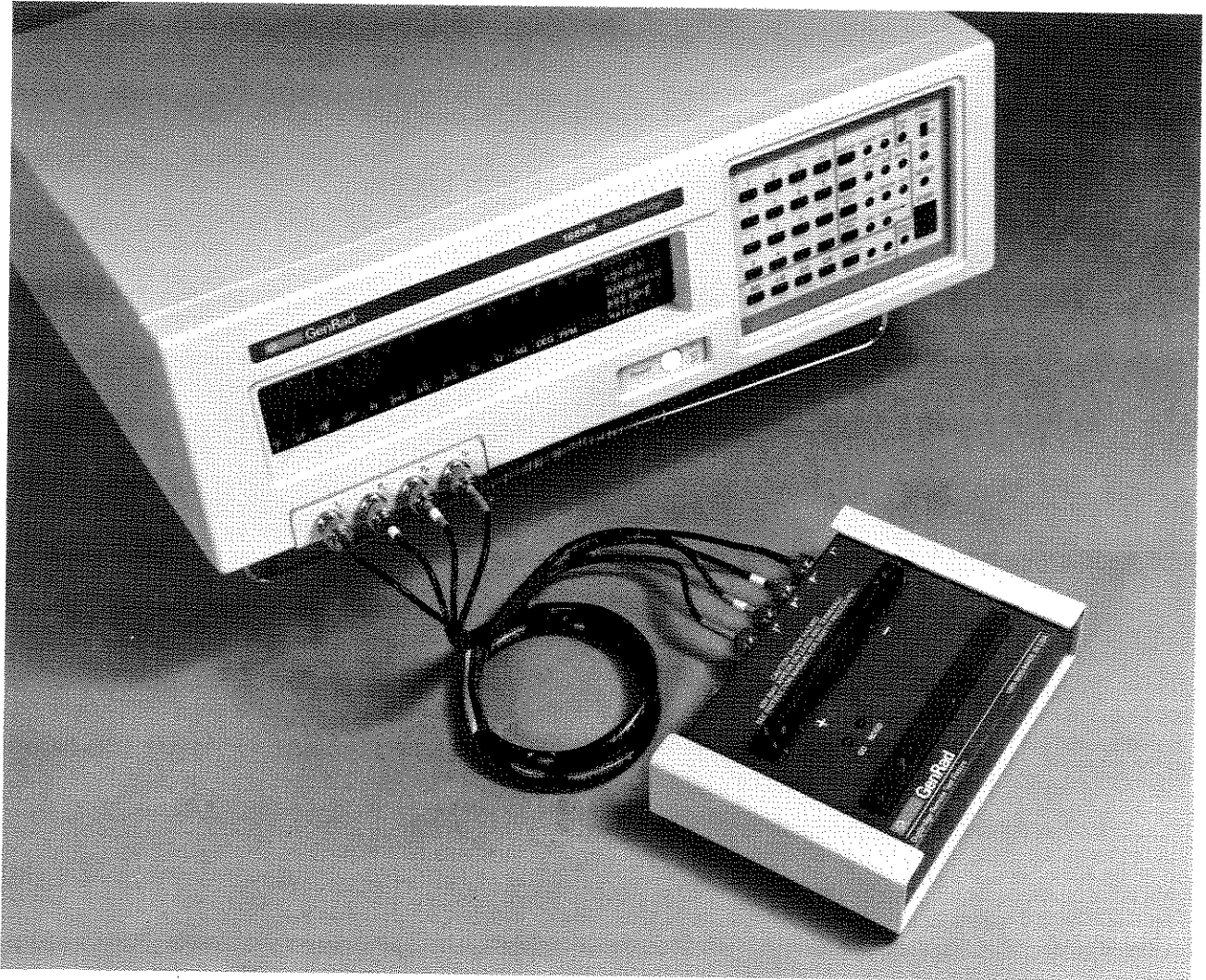
Figure 3-1. Remote test fixture (1689-9605), connected to 1689-9751 Digibridge tester.
