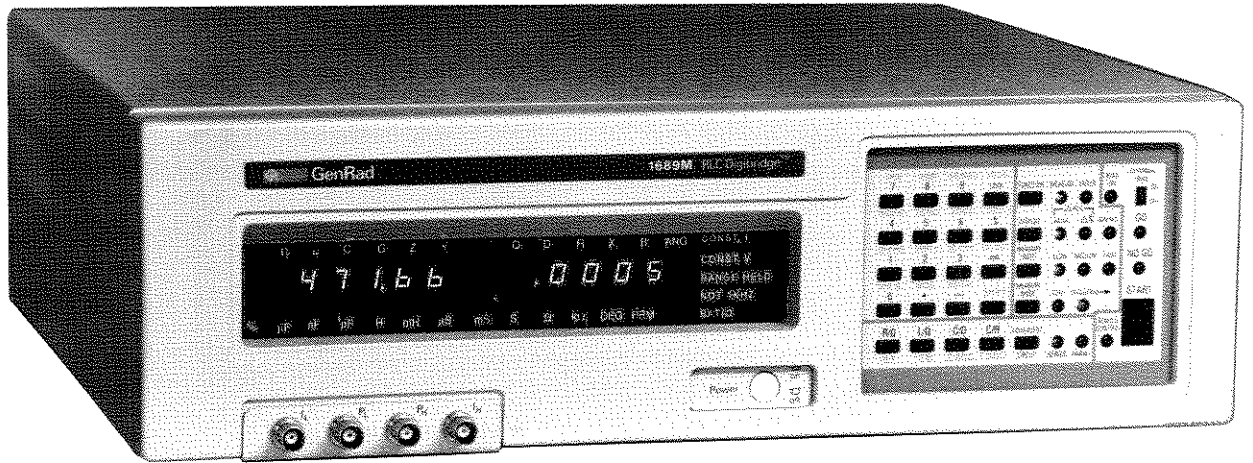
Figure 1-1. The 1689-9751 RLC DigiBridge tester, front view.
