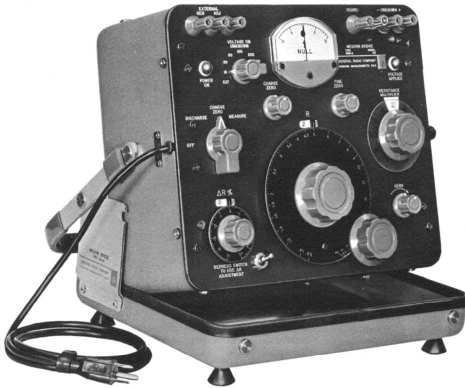
Figure 1-1. The Type 1644-A Megohm Bridge. The convenient Flip-Tilt case provides protection during transport and storage and holds open at any convenient viewing angle.
