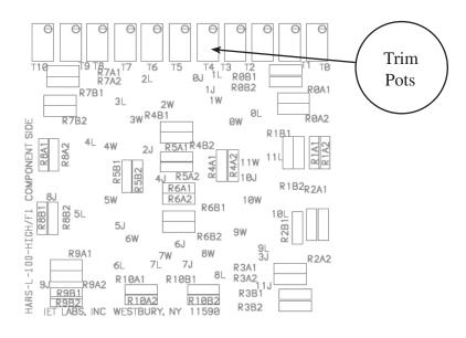
Figure 5-1: Typical Trimmer Board
