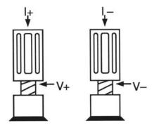
Figure 3.1 Optimal 4-Wire Kelvin Lead Connection
