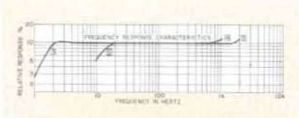
Response characteristics for constant applied (1) acceleration, (2) jerk, (3) velocity, (4) displacement, 2-Hz cutoff, and (5) displacement, 20-Hz cutoff.
