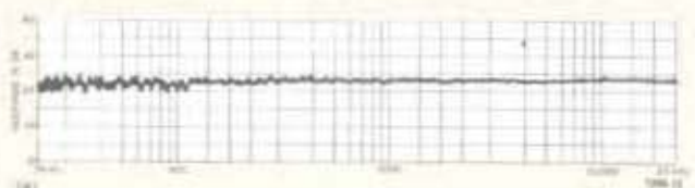
(A) Output (white noise) of the 1390-B Random-Noise Generator and (B) output (pink noise) after filtering by the 1390-P2 Pink-Noise Filter, as measured by a one-third-octave band analyzer.
