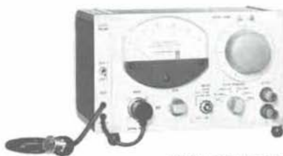
1232-P2 Preamplifier installed.
