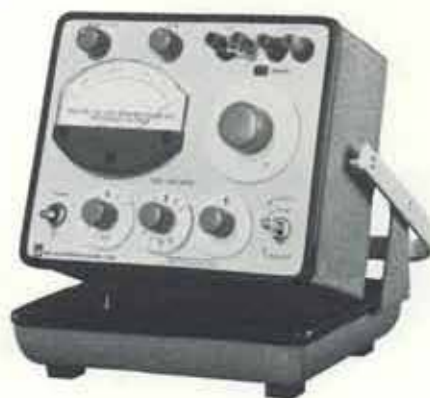
Flip-Tilt case in one of its many operating positions. Rubber gasket provides friction to allow almost any tilt angle.
