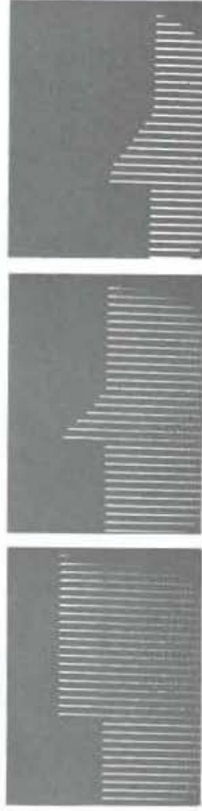
Oscillograms of line-voltage peaks show response speed of Variac® automatic voltage regulators: left, 2% step change in line voltage; center and right, resulting output transients for 1581 and 1582 Regulators, respectively.
