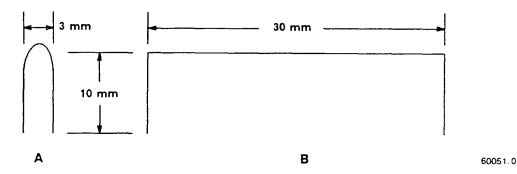
Figure 3-11. Shapes of wire recommended for short-circuit zeroing procedures before critical low-impedance measurements. Use "A" for radial-lead or miscellaneous DUTs. Use "B" before installing adaptors for axial-lead DUTs.
