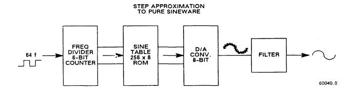
Figure 4-4. Sine wave generator. Given square waves at frequencies of 64 f, 32 f, 16 f, 8 f, 4 f, 2 f, and f, a ROM containing the mathematical sine function drives a D/A converter to form a finely stepped approximation to a sine wave at frequency f. The filter provides smoothing of the test signal.
