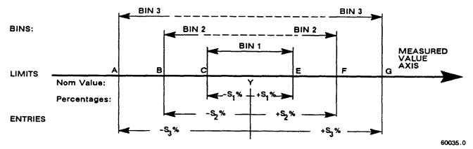
Figure 3-12. Nested limits. A single nominal value Y is used and all limit pairs are symmetrical in this basic plan.
