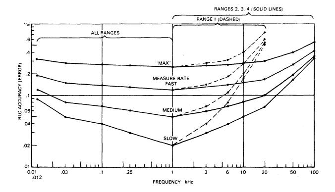
Figure 3-10. Approximate RLC accuracy vs test frequency for these test conditions: R, L, and C within basic range< D< <lor Q> >1, test voltage => 1 V, constant voltage NOT selected. The curves are labeled according to measure rate, SLOW, MEDnJM, and FAST; "Max" is FAST with integration-time factor set to 0.25 (a special function).
