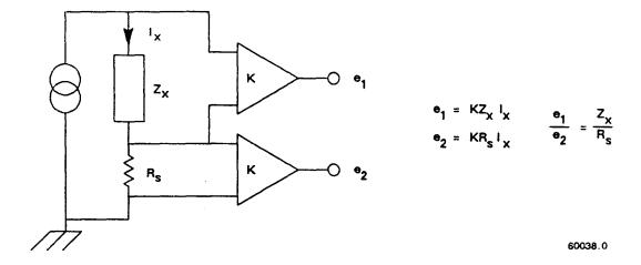
Figure 4-2. Elementary measurement circuit.
