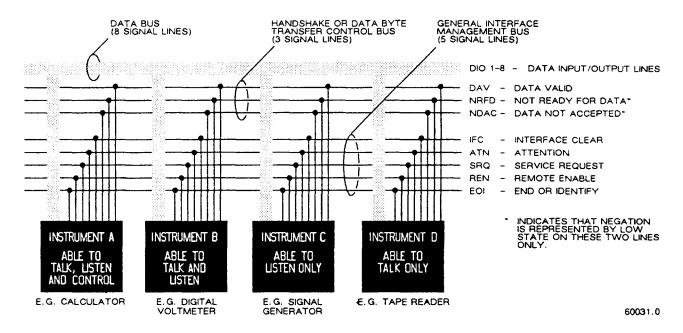
Figure 2-4. Block diagram of a generalized system interconnected by the 16-signal- line bus specified in the IEEE Standard 488. Reprinted from *Electronics*, November 14, 1974; copyright McGraw-Hill, Inc., 1974.
