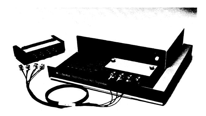
Figure 3-4. Remote test fixture (1689-9600), connected to 1689 Digibridge tester.
