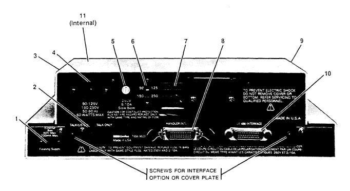
Figure 1-3. Rear controls and connectors, 1689 Digibridge.
