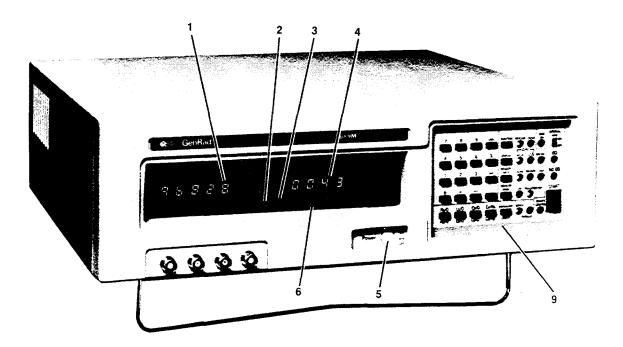
Figure 1-1. The 1689M RLC Digibridge tester, front view.
