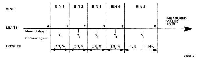
Figure 3-13. Sequential limits. A different nominal value is entered for each bin and all limit pairs are symmetrical except for the unsymmetrical pair shown for example in bin 5.
