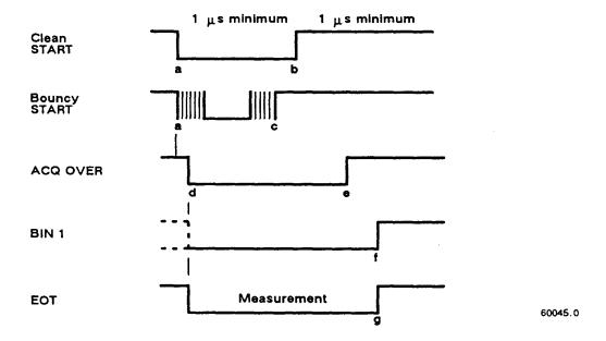
Figure 2-3. Handler interface timing diagram. External circuit must keep a-b > 1 us, and (if START is not "debounced") a-c < [the settling time or programmed delay]. For single measurements, the DUT can be disconnected after e. The selected BIN line goes low at f; the other BIN lines stay high. For MEDIAN and/or AVERAGE measurement routines, ACQ OVER goes low (e) at the end of the last measurement.
