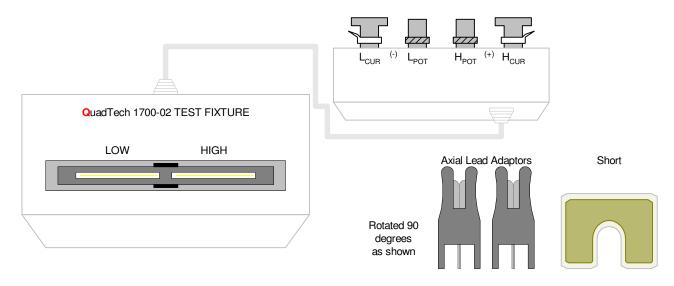
Figure A-2: 1700-02 Axial/Radial Remote Test Fixture
