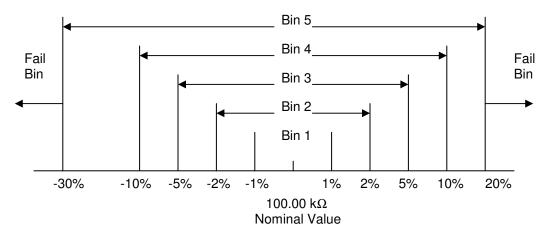
Sequential limits are a natural choice for sorting by absolute value. Sequential limits for four bins are illustrated below. It should be noted that the bins do not necessarily have to be adjacent. Depending on the specified limits for each they can be overlapping, adjacent or even isolated (gaps) from each other. Any overlap is assigned to the lower numbered bin and a gap would be assigned to the overall fail bin.
