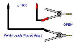
Press the [START] to initiate open calibration measurement
