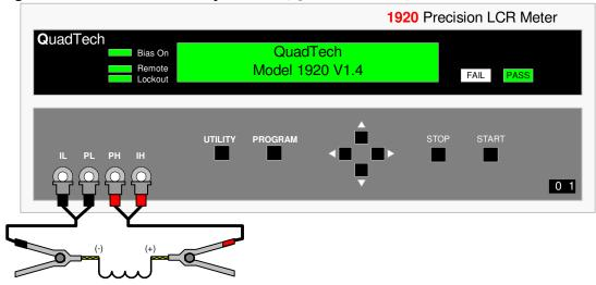
Figure COI-1: Connection to DUT using 1700-03 Kelvin Leads
