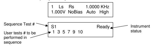
The above display is typical showing S1 is the sequence test setup #, the sequence programmed to perform user tests 1,3,5,7,9,and 10 in succession, and Ready the instrument status. To select any other sequence test number simply press the Up or Down arrow keys while in the Ready state.
