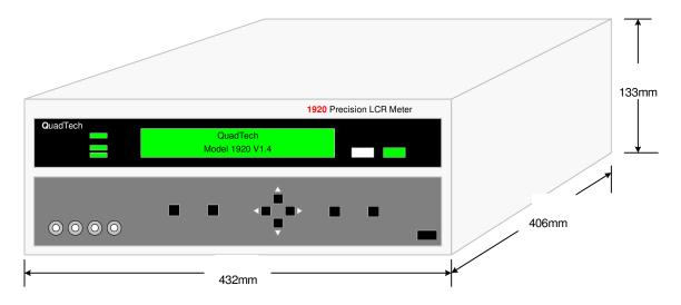
**Figure 1-3: Instrument Dimensions**
