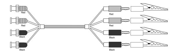
Figure A-4: 1700-04 BNC (4) Connectors to Banana Plugs (4)
