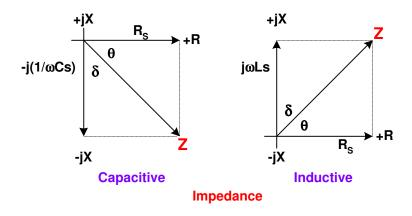
Figure 2-3a Phase Diagrams of Impedances
