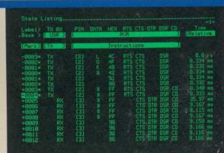
Figure 2 — The sequence LOKB was found. Transmitted and received data, and control functions are displayed along with their respective input pin numbers. The HP 1630G also shows the actual elapsed time between states. Note the bus turn-around time when changing from transmit to receive.
