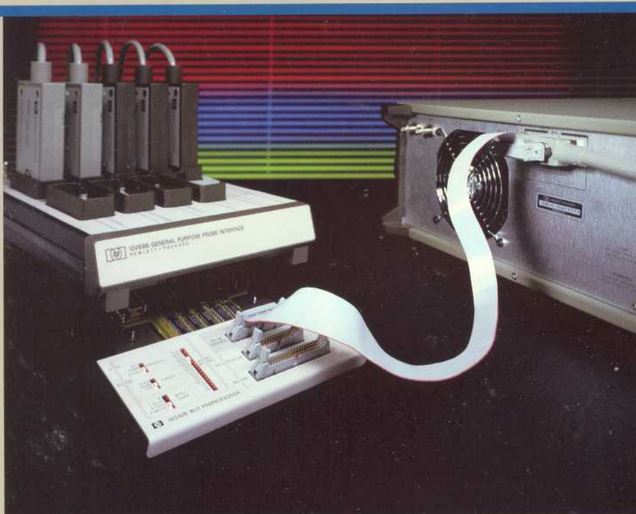
The HP 10342B bus preprocessor connects to the HP 10269B general-purpose probe interface for direct and non-intrusive monitoring of HP-IB, RS-232C/V.24, and RS-449.
