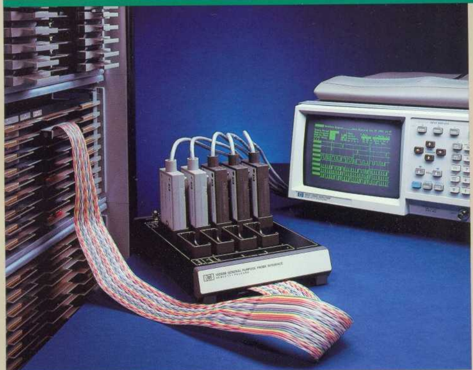
Interfacing to minicomputers is simplified with HP's minicomputer interfaces or with the HP 10320A and HP 10321A user-definable modules.
