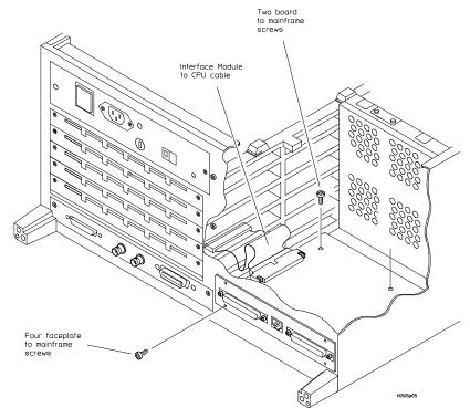
**Removing the Interface Module**
