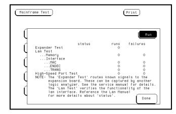
If an HP 16501A expansion frame is not connected, then expect a "No Expansion Card Present" message to appear when you run the Option Board Test. Refer to the *HP 16500B/16501A Service Guide* for more information about the expansion frame.
