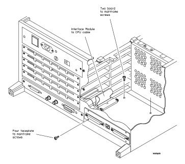
Installing the Interface Module
