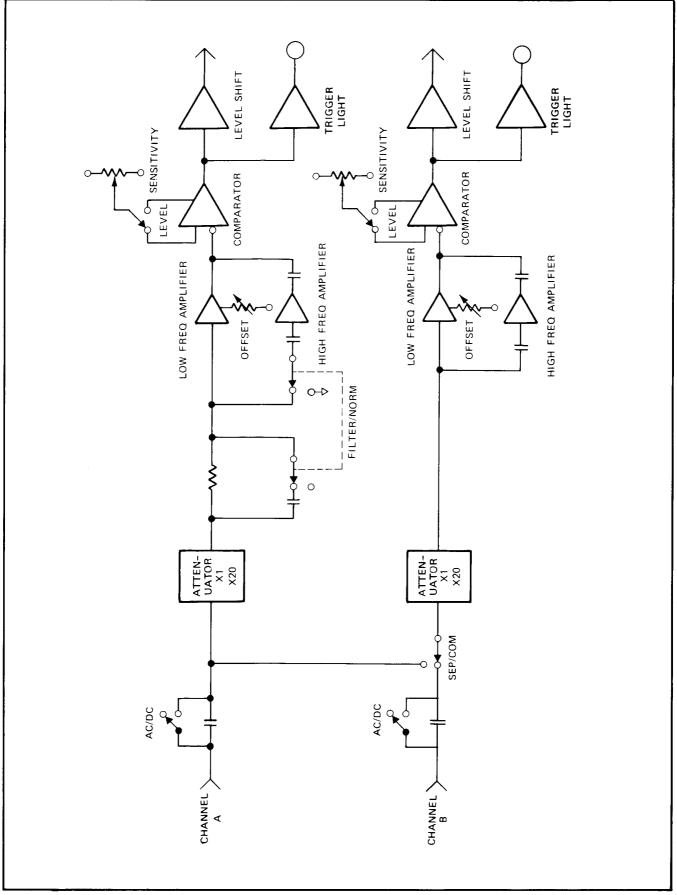
Figure 3-6. 5315A/B Front End Block Diagram
