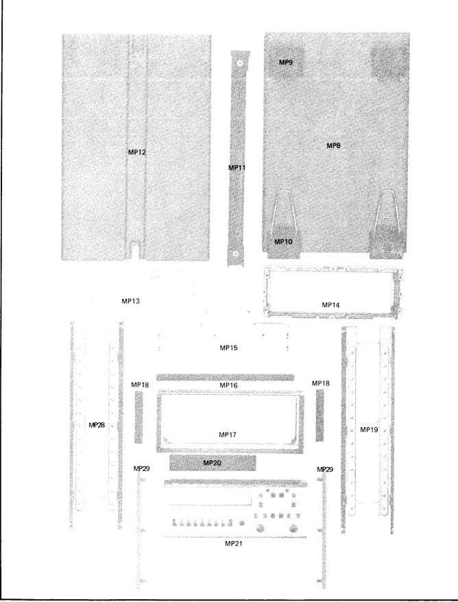
Figure 6-2. Model 5315B Mechanical Parts Layout
