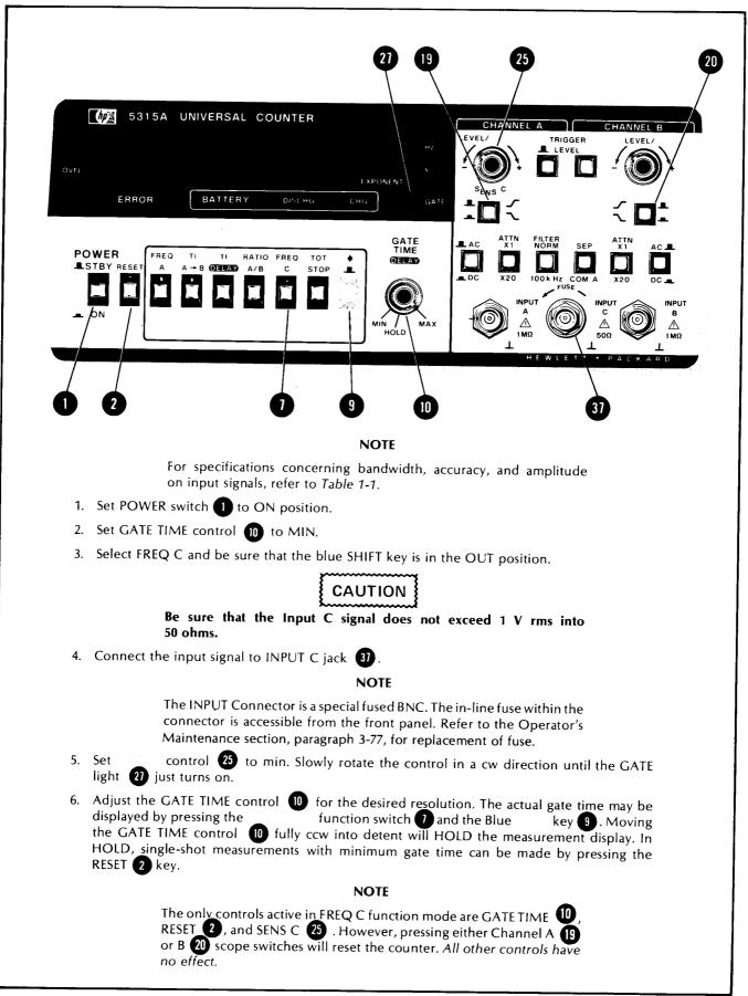
Figure 3-21. Frequency C Measurement (Option 003)
