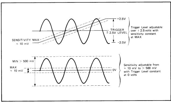
Figure 3-5. Trigger Level/Sensitivity Controls
