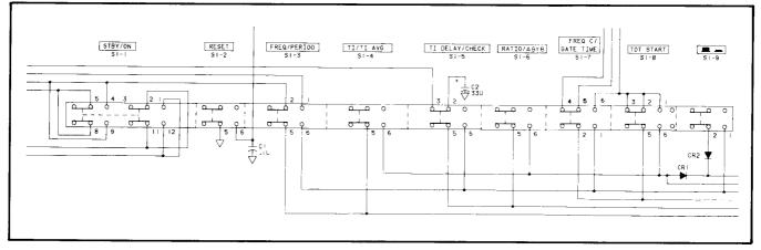
Figure 7-2. A1S1 Switch Assembly (A1 Assembly Series 1928)
