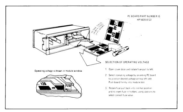
Figure 2-2. 5315B Line Voltage Selection Card
