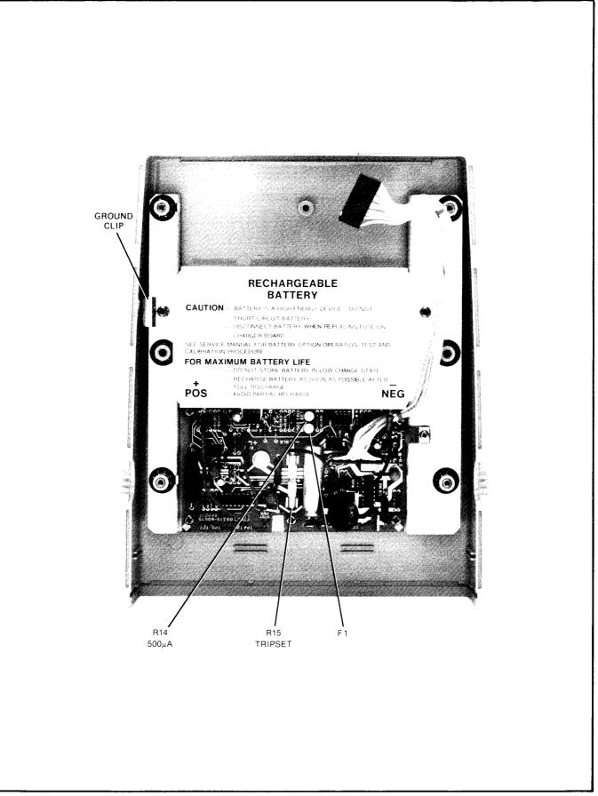
Figure 5-4. Option 002 Battery Charger Adjustment Locations
