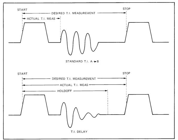
Figure 3-2. Timing of Time Interval Delay Mode
