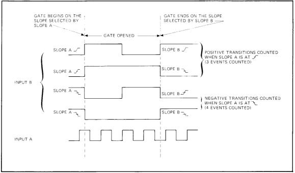
Figure 3-3. Timing of Totalize A by B Mode
