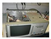
Once the top cover removed, complex electronics are discovered. The power supply is in the air flow of the fan, which is its place. Against the left wall is the control and power of the CRT, and the bottom of the deck housing management occupies the entire space.
