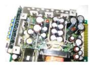
For secondary side. Not bad capacitors, large cooled chokes and diodes: this gives more power voltages for different parts of the device. But it is also, curiously, classic LM350 regulators and MOS transistors on a heatsink. Only the statement of the scheme will help to understand ...
