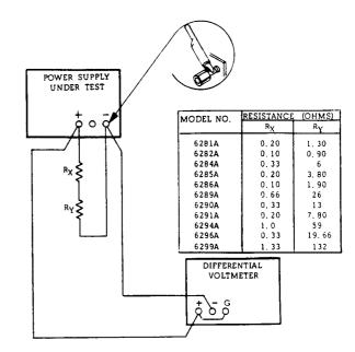
Figure 5-5. Load Regulation, Constant Voltage
