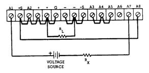
Figure 3-6. Remote Voltage Programming (Constant Current)
