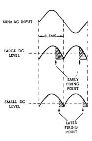
Figure 4-3. SCR Phase Control of DC Input Level
