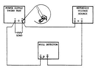
Figure 5-3. Differential Voltmeter Substitute, Test Setup
