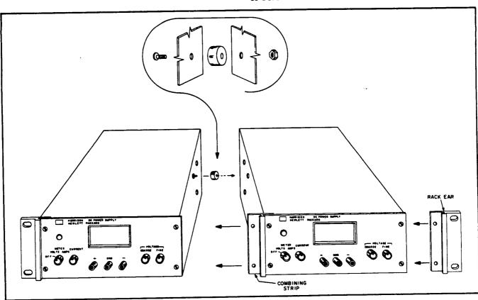
Figure 2-1. Rack Mounting, Two Units
