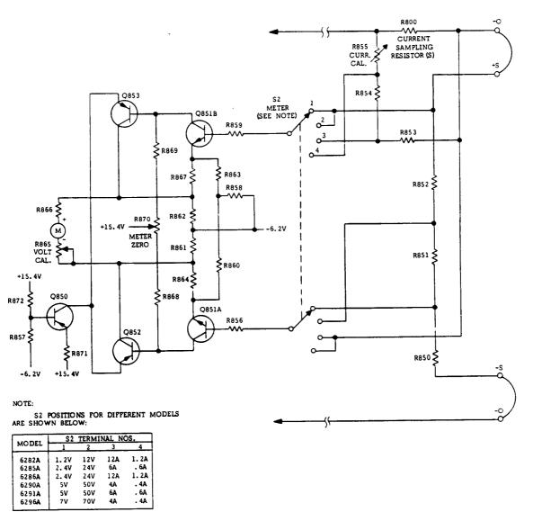
Figure 4-8. Meter Circuit, Simplified Schematic
