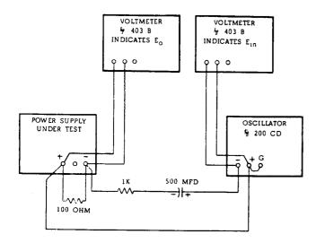
Figure 5-9. Output Impedance, Test Setup
