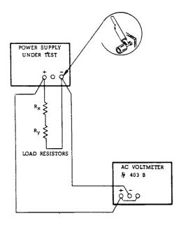
Figure 5-6. Ripple and Noise, Constant Voltage
