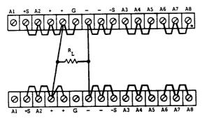
Figure 3-10.\ Normal Parallel Connections
