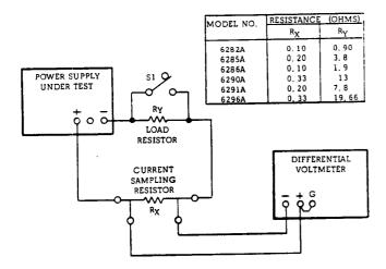
Figure 5-4. Output Current Test Setup
