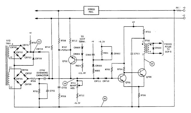
Figure 4-4. SCR Control Circuit, Simplified Schematic
