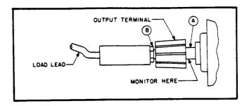
Figure 5-1. Front Panel Terminal Connections
