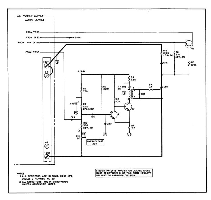
Figure A-1. Model 6286A Overvoltage Protection Crowbar
