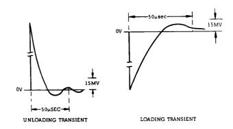
Figure 5-8. Transient Response Waveforms
