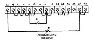
Figure 3-5. Remote Resistance Programming (Constant Current)
