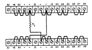
Figure 3-8. Normal Series Connections
