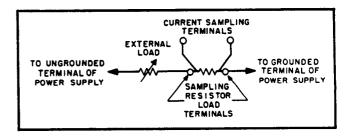
Figure 5-2. Output Current Measurement Technique
