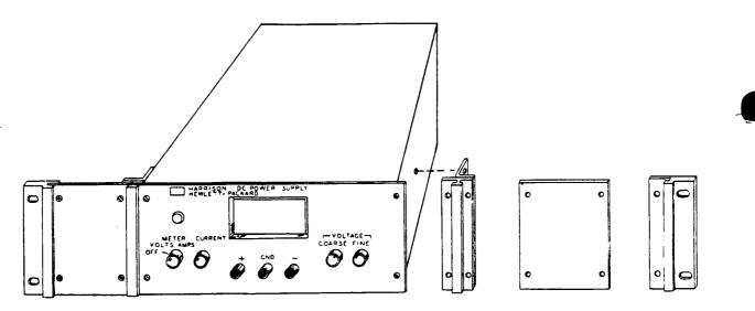
Figure 2-2. Rack Mounting, One Unit
