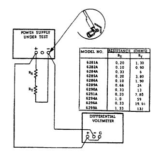
Figure 5-5. Load Regulation, Constant Voltage
