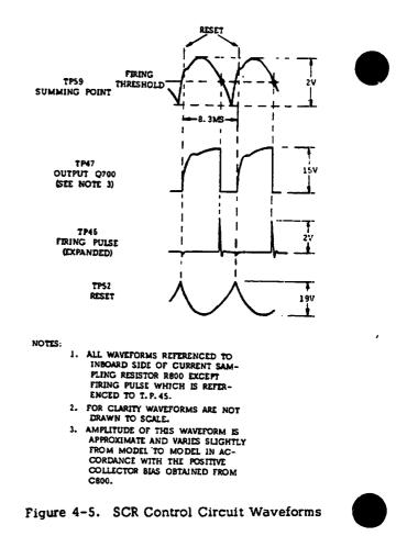
diagram. The firing pulse is relatively narrow because Q700 saturates rapidly causing the magnetic field surrounding T700 to collapse. Diode CR500 damps out the negative overshoot.
