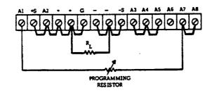
Figure 3-5. Remote Resistance Programming (Constant Current)
