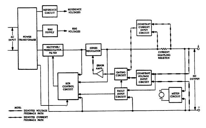
Figure 4-1. Overall Block Diagram
