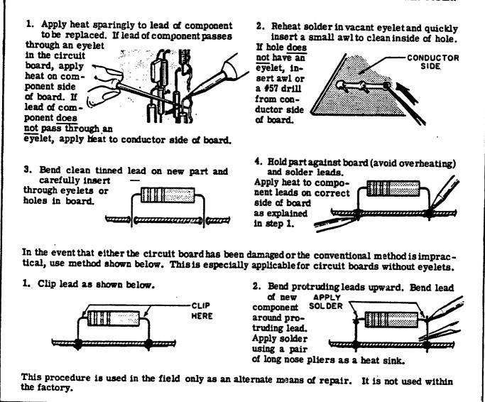
Figure 5-10. Servicing Printed Wiring Boards
