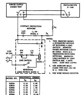
Figure 5-7. Transient Response, Test Setup
