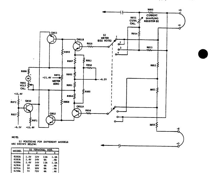
Figure 4-8. Meter Circuit, Simplified Schematic
