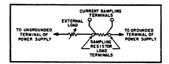
Figure 5-2. Output Current Measurement Technique
