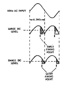
Figure 4-3. SCR Phase Control of DC Input Level
