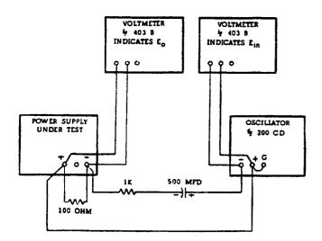
Figure 5-9. Output Impedance, Test Setup
