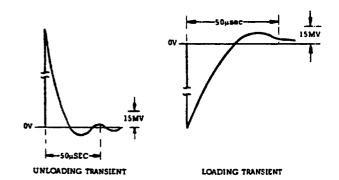
Figure 5-8. Transient Response Waveforms
