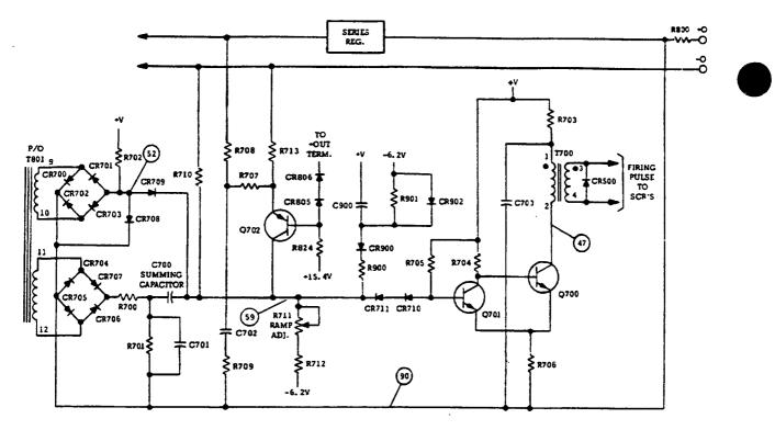
Figure 4-4. SCR Control Circuit, Simplified Schematic
