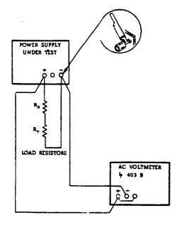
Figure 5-6. Ripple and Noise, Constant Voltage
