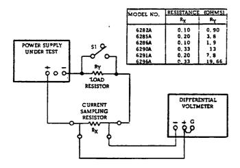
Figure 5-4. Output Current Test Setup
