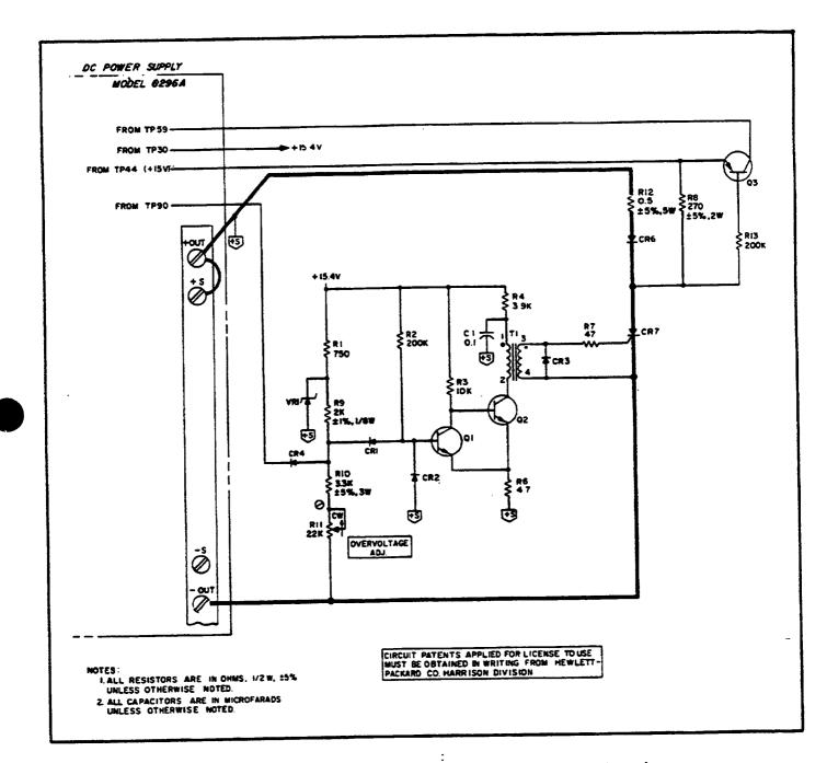
Figure A-1. Model 6296A Overvoltage Protection Crowbar
