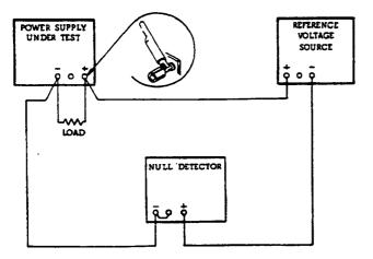
Figure 5-3. Differential Voltmeter Substitute, Test Setup
