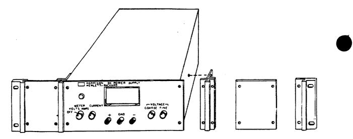
Figure 2-2. Rack Mounting, One Unit
