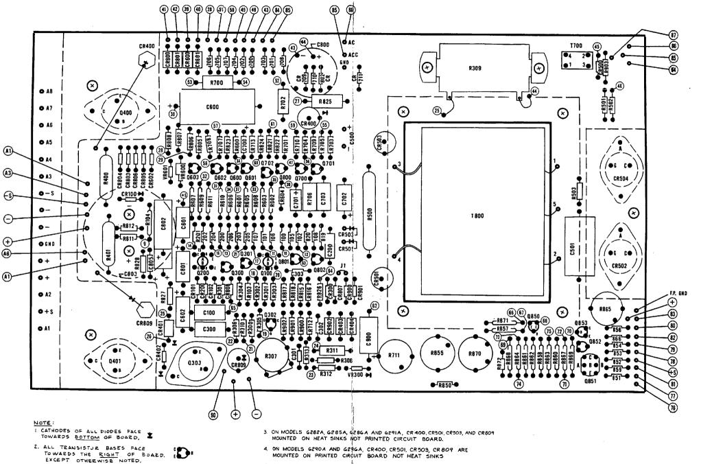
5. ON MODELS G285A, G290A, G291A, AND G29GA, R401 AND Q401 ARE NOT USED AND R400 IS REPLASED WITH A JUMPER
