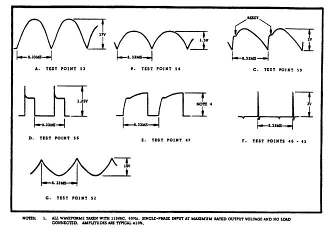
2. OSCILLOSCOPE DC COUPLED AND REFERENCED TO T. P. 90 UNLESS OTHERWISE INDICATED.
