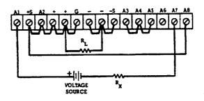
Figure 3-6. Remote Voltage Programming (Constant Current)
