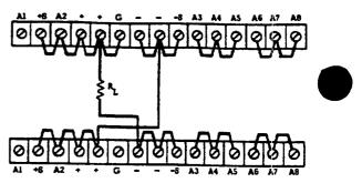
Figure 3-8. Normal Series Connections
