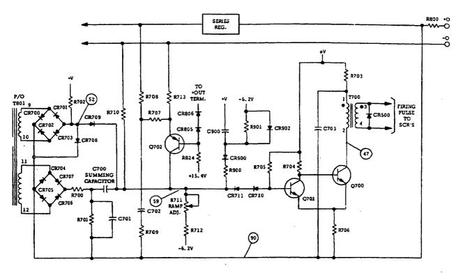
Figure 4-4. SCR Control Circuit, Simplified Schematic
