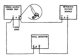
Figure 5-3. Differential Voltmeter Substitute, Test Setup
