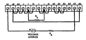
Figure 3-6. Remote Voltage Programming (Constant Current)
