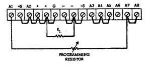
Figure 3-5. Remote Resistance Programming (Constant Current)
