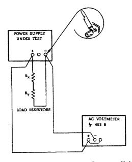
Figure 5-6. Ripple and Noise, Constant Voltage
