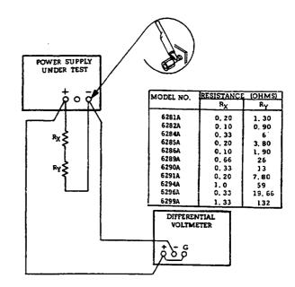
Figure 5-5. Load Regulation, Constant Voltage
