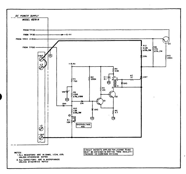
Figure A-1. Model 6291A Overvoltage Protection Crowbar
