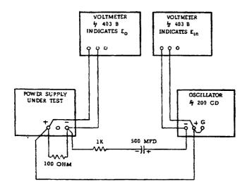
Figure 5-9. Output Impedance, Test Setup
