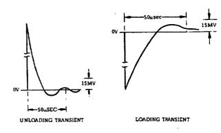
Figure 5-8. Transient Response Waveforms
