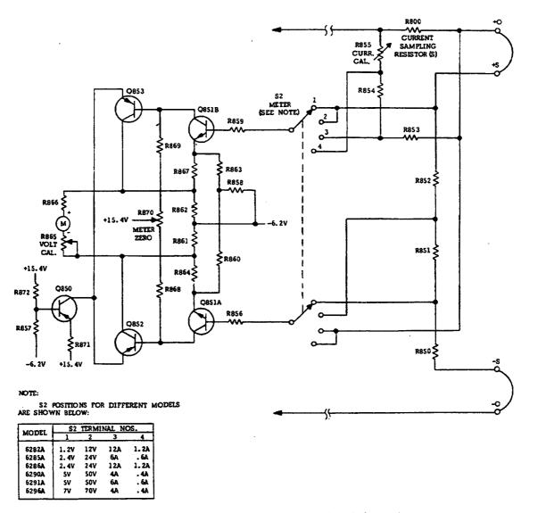
Figure 4-8. Meter Circuit, Simplified Schematic
