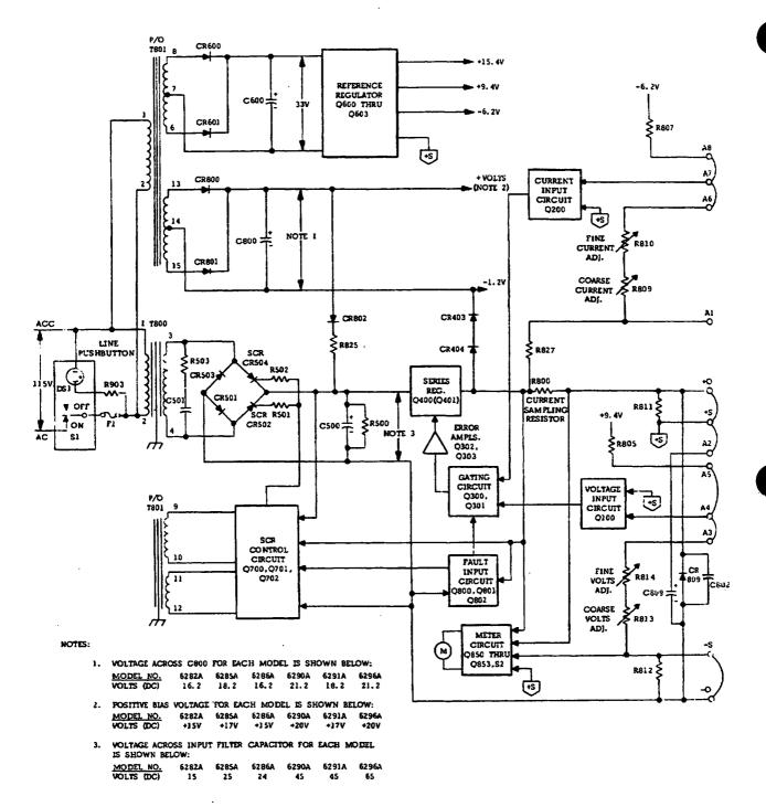
Figure 4-2. Simplified Schematic
