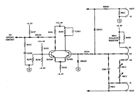
Figure 4-6. Constant Voltage Input Circuit, Simplified Schematic
