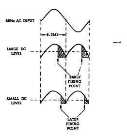
Figure 4-3. SCR Phase Control of DC Input Level
