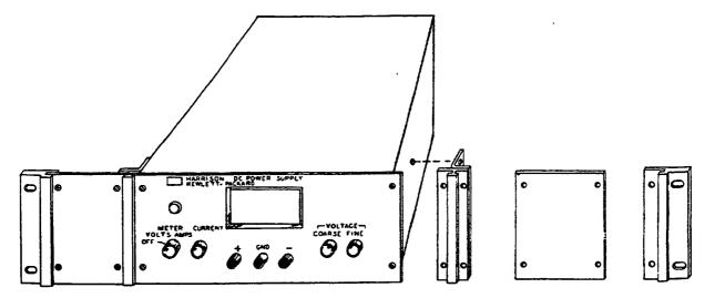
Figure 2-2. Rack Mounting, One Unit
