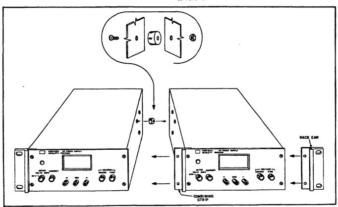
Figure 2-1. Rack Mounting, Two Units
