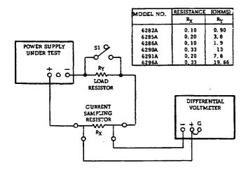
Figure 5-4. Output Current Test Setup
