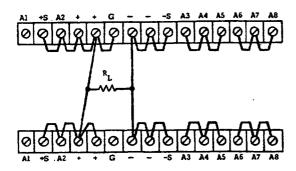
Figure 3-10. Normal Parallel Connections
