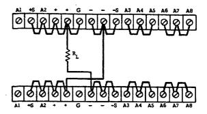
Figure 3-8. Normal Series Connections
