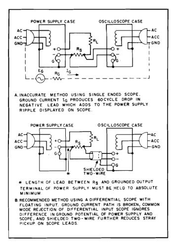
Figure 5-8. Constant-Current Ripple and Noise Test Setup
