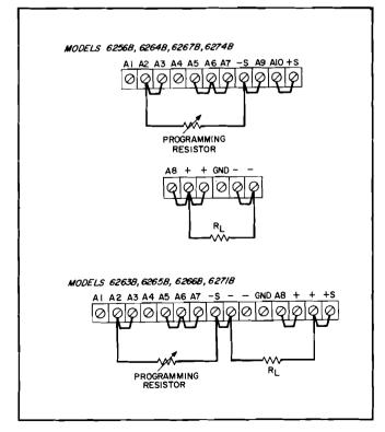
Figure 3-4. Resistance Programming of Output Voltage
