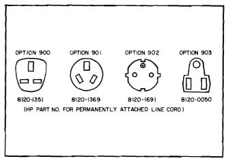
Figure 2-4. Power Cord Configurations
