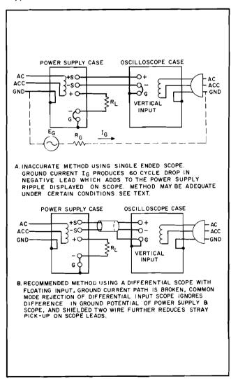
Figure 5-2. Ripple Test Setup
