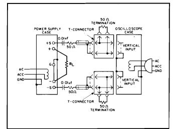
Figure 5-3. Noise Spike Measurement Test Setup
