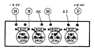
Figure 7-2. Option 020, 021, 022, 040 Circuit Board Component Locations
