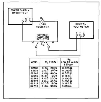
Figure 5-7. Constant-Current Load Regulation Test Setup
