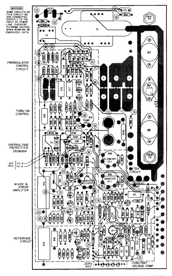
Figure 7-3. A1 Board Component Locations for Models 6256B, 6264B, 6267B, and 6274B
