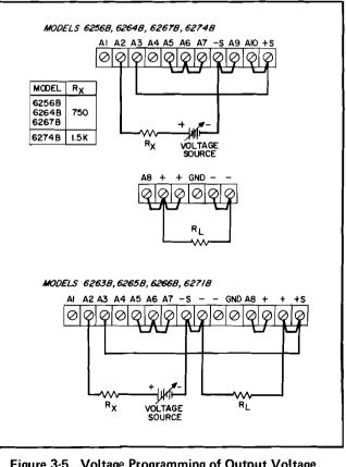
Figure 3-5. Voltage Programming of Output Voltage (Unity Gain)
