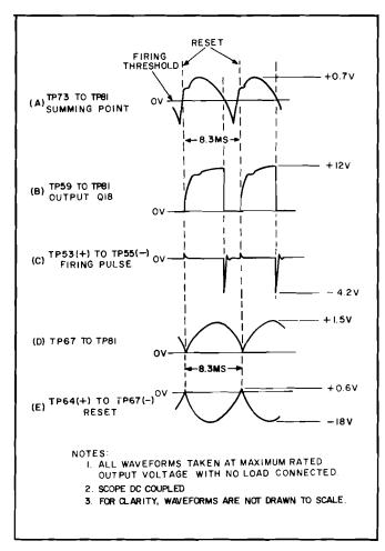
Figure 4-4. Preregulator Control Circuit Waveforms
