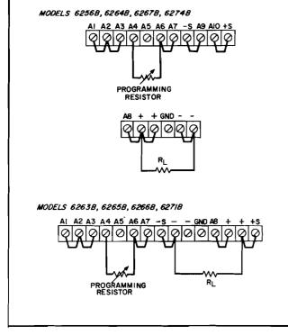
Figure 3-6. Resistance Programming of Output Current
