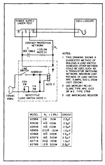
Figure 5-4. Load Transient Recovery Time Test Setup
