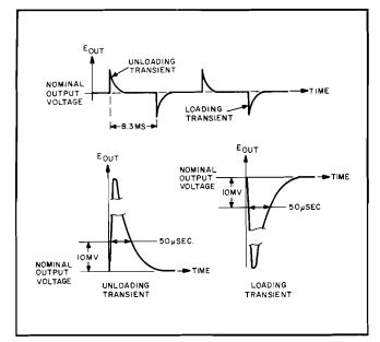
Figure 5-5. Load Transient Recovery Time Waveforms
