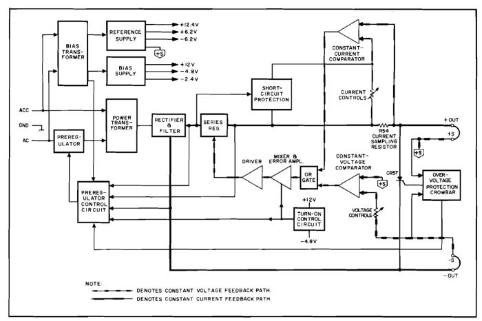
Figure 4-1. Overall Block Diagram
