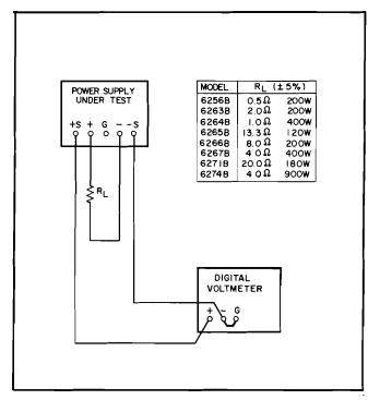
Figure 5-1. Constant-Voltage Load Regulation Test Setup
