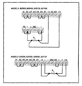
Figure 3-3. Remote Sensing
