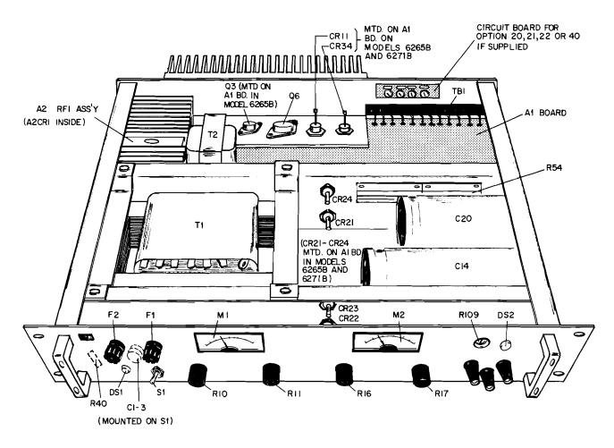
Figure 7-8. Chassis Component Locations for Models 6263B, 6265B, 6266B, and 6271B
