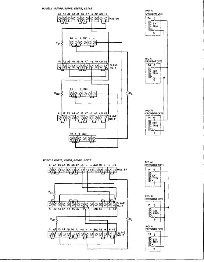
Figure 3-11. Auto-Series Operation of Three Units
