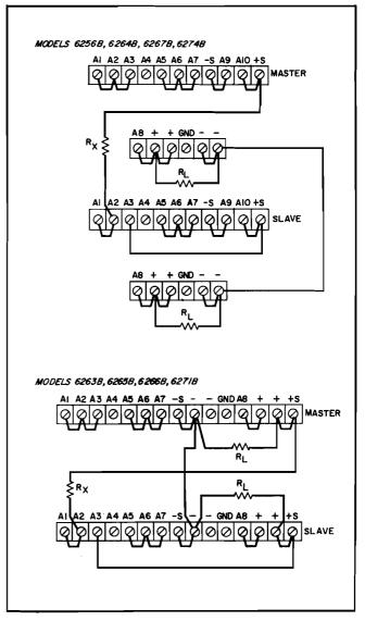
Figure 3-12. Auto-Tracking Operation of Two Units
