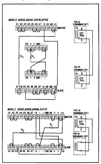
Figure 3-10. Auto-Series Operation of Two Units
