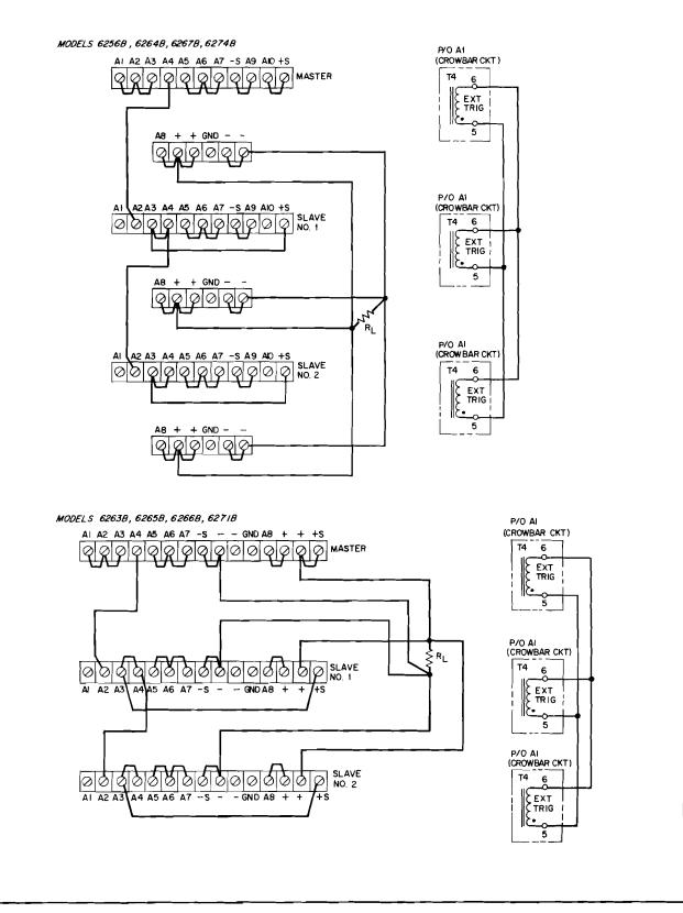
Figure 3-9. Auto-Parallel Operation of Three Units
