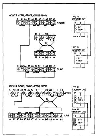
Figure 3-8. Auto-Parallel Operation of Two Units
