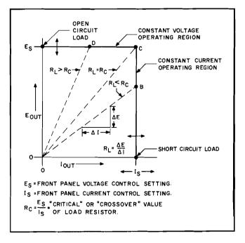
Figure 4-2. Operating Locus of a CV/CC Power Supply
