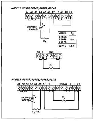
Figure 3-7. Voltage Programming of Output Current
