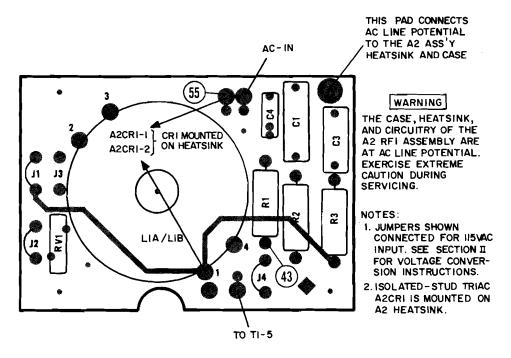
Figure 7-1. A2 RFI Assembly Component Locations
