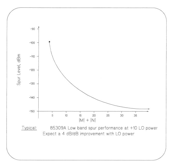
Figure 1. Spur Level Performance in Low Band
