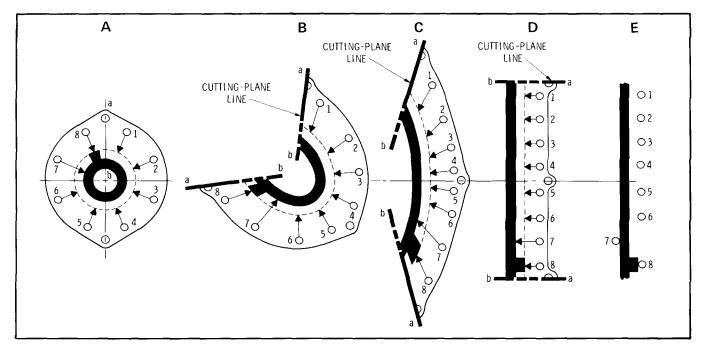
Figure 8-5. Evolution of Straight-Line Switch Presentation
