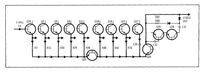
Figure 8-35. Simplified Diagram - Log Mode of Operation
