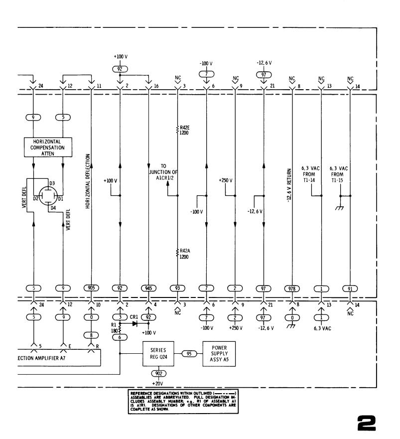
Figure 8-14. RF Section/IF Section/Display Section Interconnections
