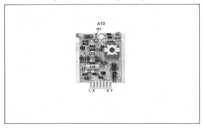
Figure 8-20. 2 MHz VTO A13 Component Identification
