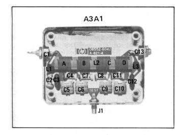
Figure 8-15. 50 MHz Bandpass Filter A3A1 Component Identification
