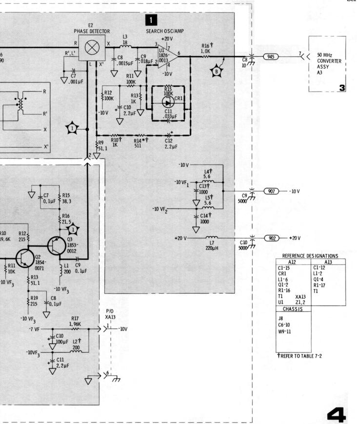
Figure 8-21. 47 MHz Automatic Phase Control and 2 MHz Voltage Tuned Oscillator
