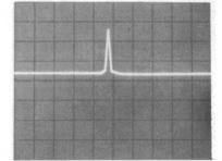
Rotate the BASE LINE CLIPPER control and observe that marker signal remains regardless of BASE LINE CLIPPER control position.
