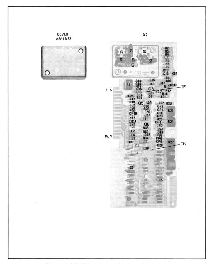
Figure 8-24. P/O 3 MHz Amplifier A2 Component Identification
