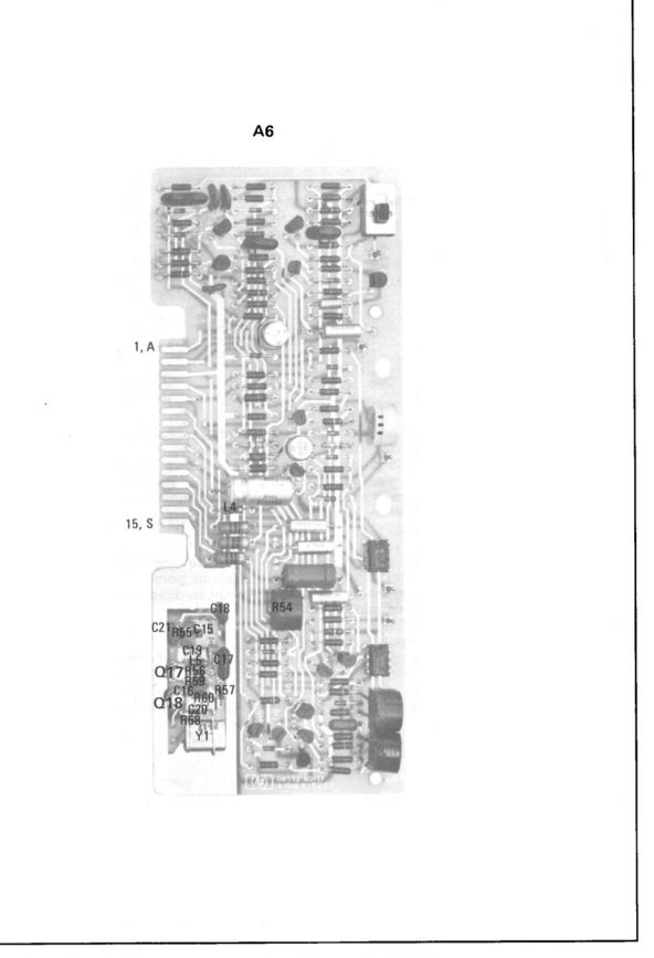
Figure 8-48. P/O Scan Generator A6 Component Identification
