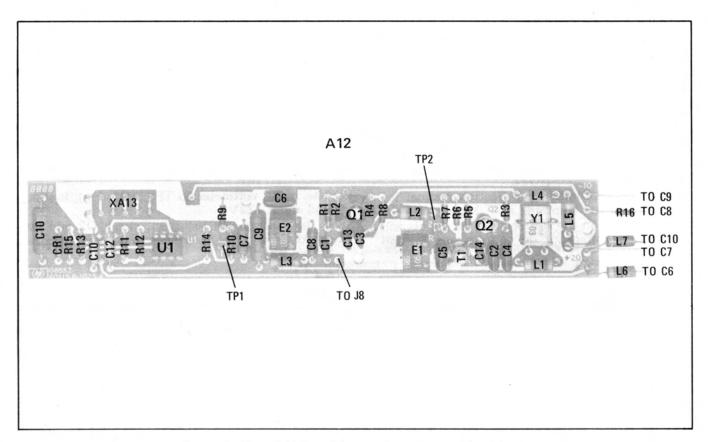
Figure 8-19. 47 MHz APC A12 Component Identification
