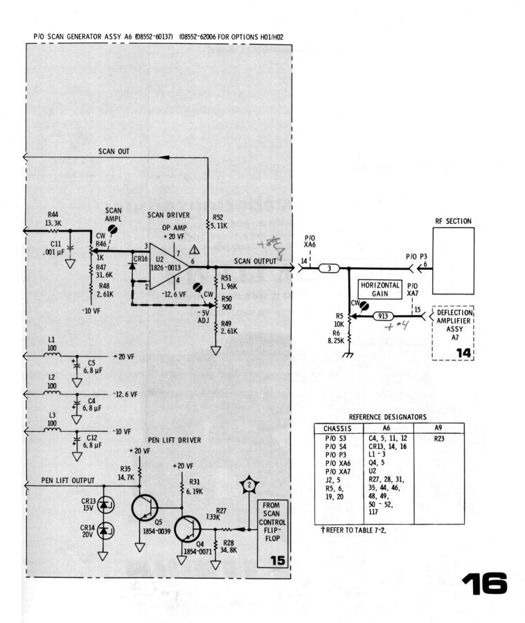
Figure 8-45. Scan Driver and Pen Lift Driver
