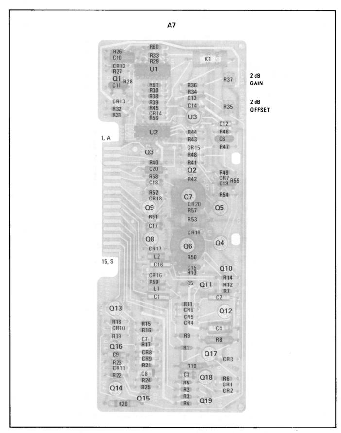
Figure 8-40. Deflection Amplifier A7 Component Identification
