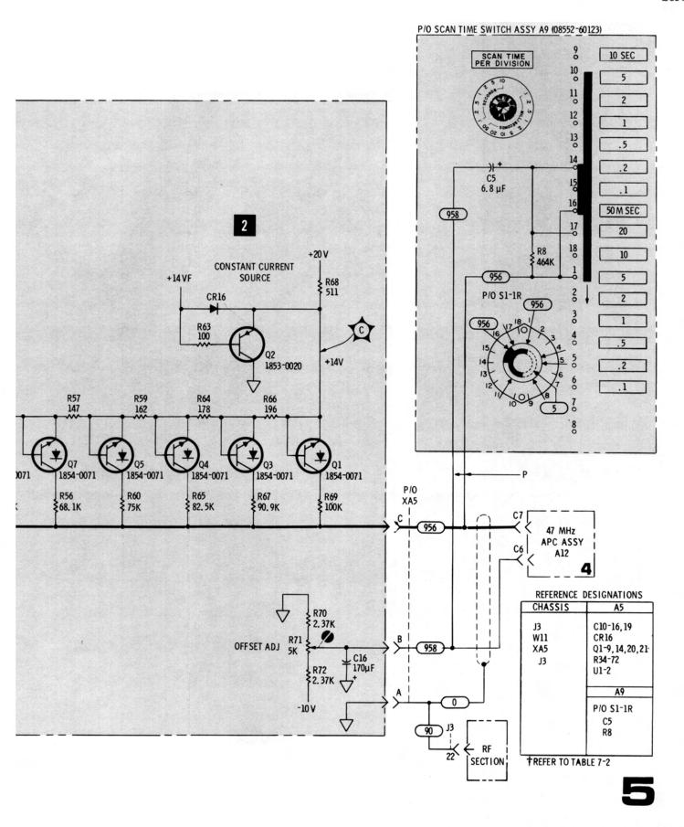
Figure 8-23. 2 MHz VTO Shaping Circuit
