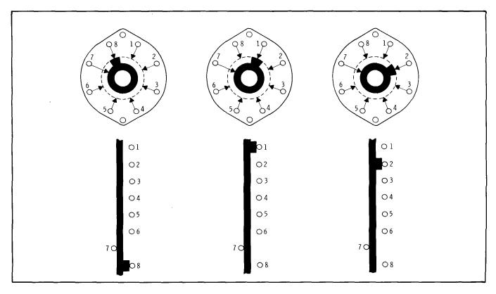
Figure 8-6. Three Positions of Typical Switch Wafers
