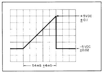
Figure 5-3. Scan Voltage Waveform Measurement
