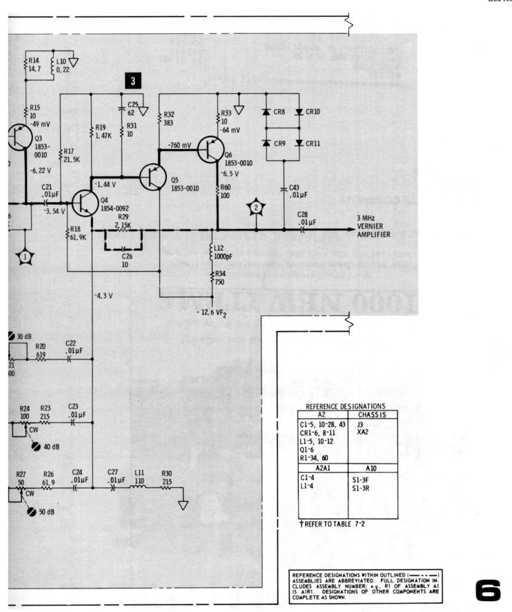
Figure 8-25. 3 MHz Amplifier (1 of 2)
