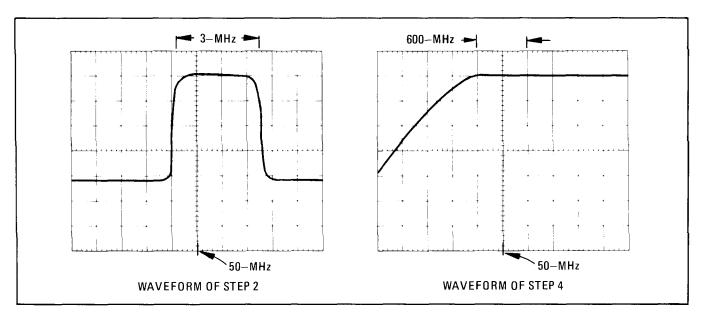
Figure 5-13. 50 MHz Bandpass Display for 10 MHz and 3 MHz Sweeps
