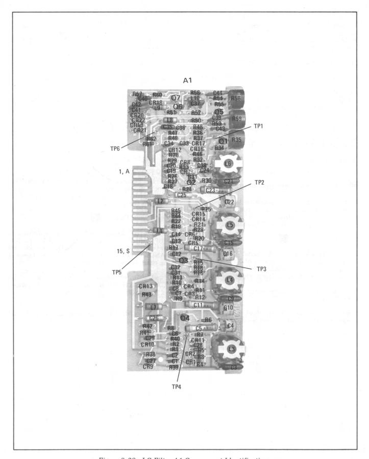
Figure 8-28. LC Filter A1 Component Identification
