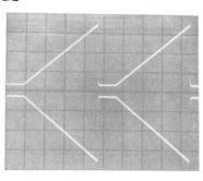
Waveform A GOOD and B BAD check Q14, 15 and associated components.
