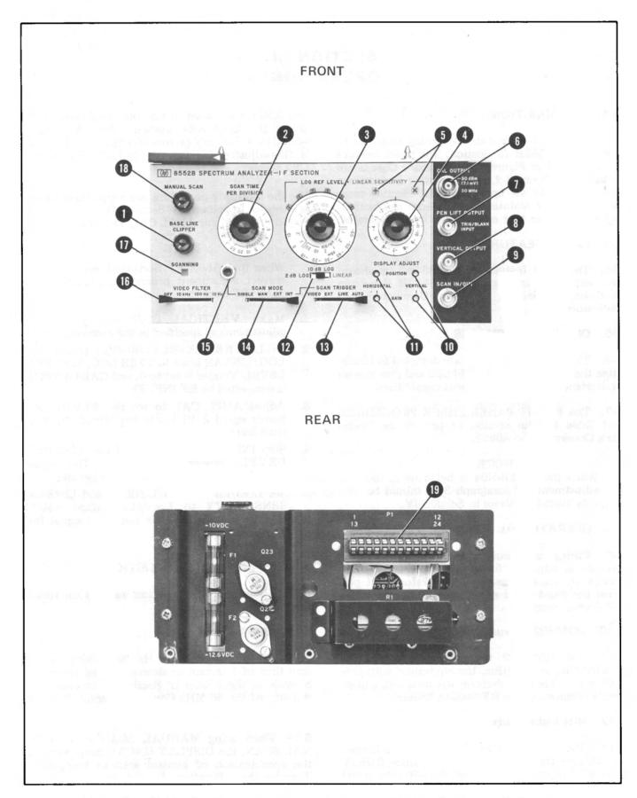
Figure 3-1. 8552B Spectrum Analyzer IF Section Controls and Connectors Indicators
