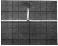
Rotate the BASE LINE CLIPPER control and observe that marker signal remains regardless of BASE LINE CLIPPER control position.
