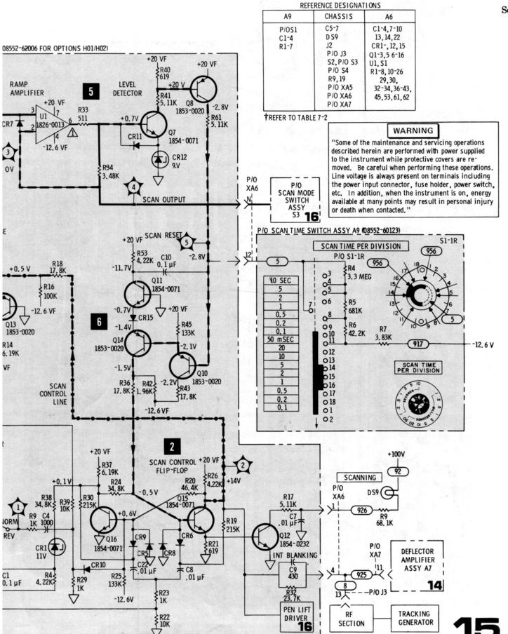
Figure 8-43. Scan Generator and Trigger Circuits
