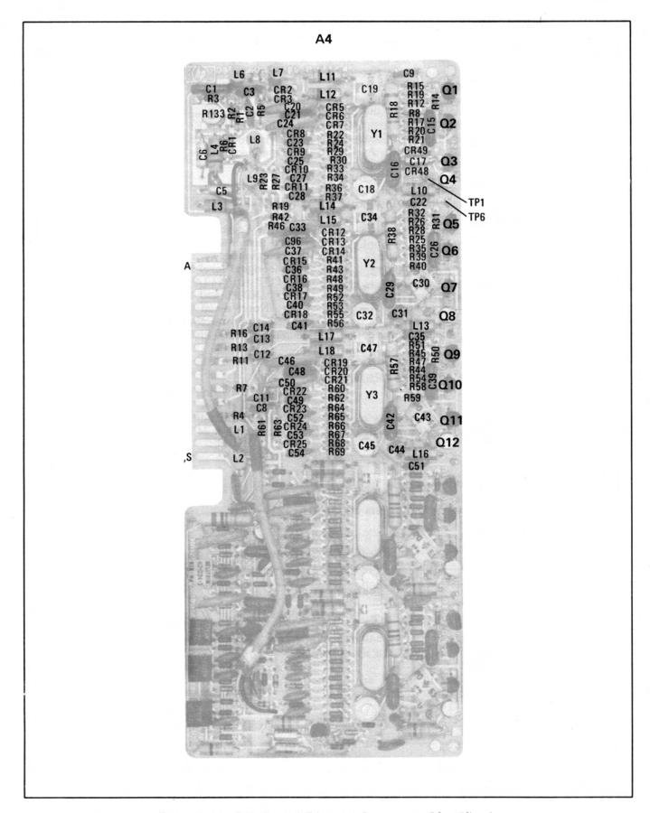
Figure 8-31. P/O Crystal Filter A4 Component Identification
