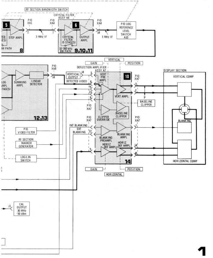
Figure 8-10. 8552B Block Diagram
