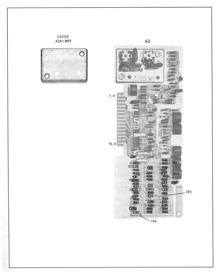
Figure 8-26. P/O 3 MHz Amplifier A2 Component Identification
