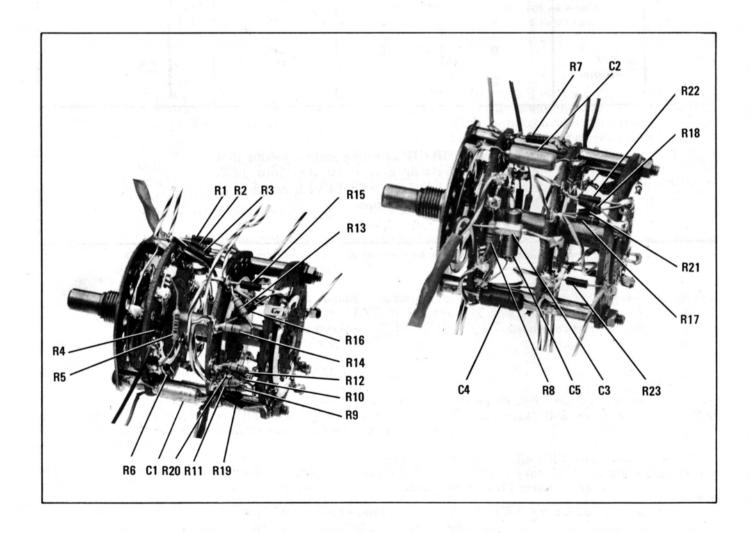
Figure 8-13. Scan Time Switch Assembly A9
