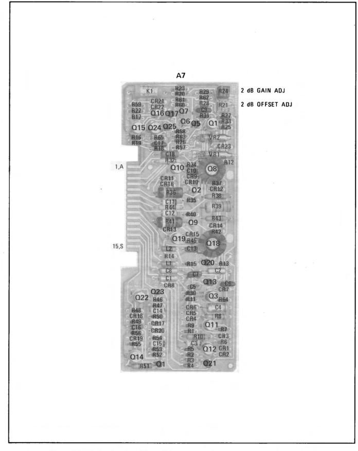
Figure 7-6. Deflection Amplifier A7 Component Identification (Part of Change O)
