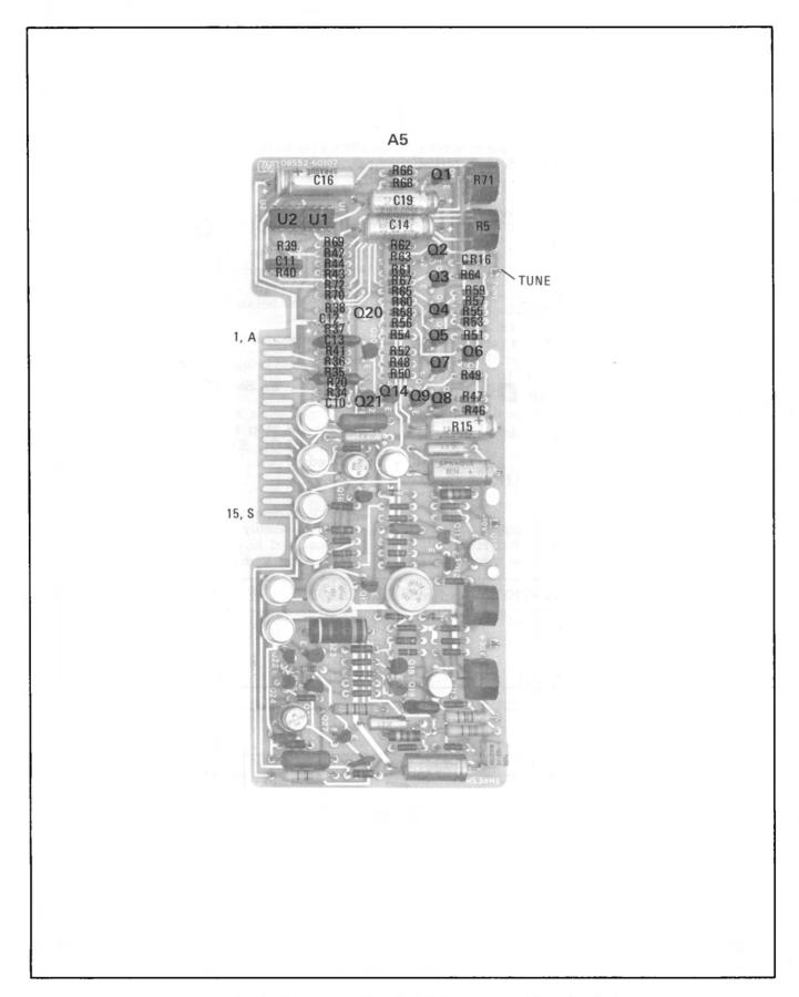
Figure 8-22. P/O Power Supply A5 Component Identification
