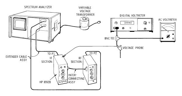
Figure 5-1. Power Supply Check and Adjustment Test Setup
