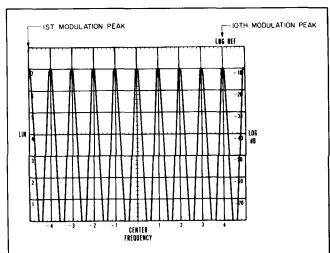
Figure 4-7. Scan Time Modulation Peaks
