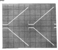
Waveform A GOOD and B BAD check Q4/Q14 and associated components.
