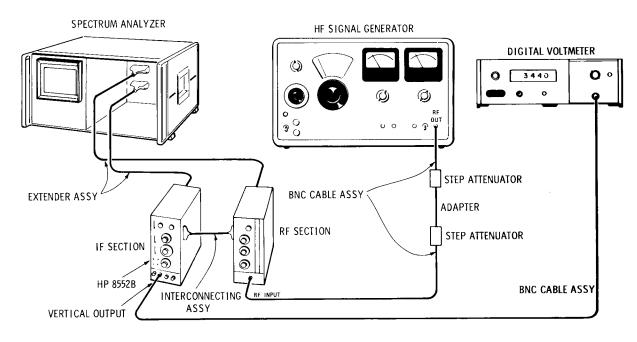
Figure 5-9. 3 MHz IF Gain Adjustment Test Setup
