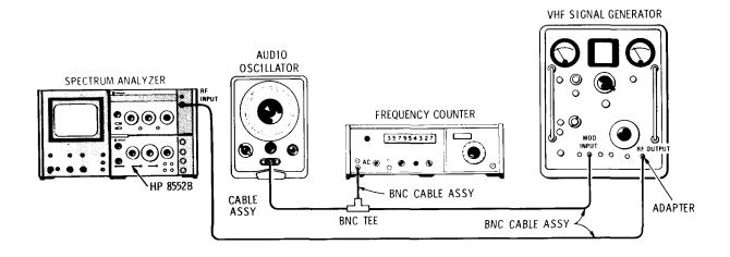
Figure 4-6. Scan Time Accuracy Test Setup
