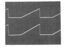
If both waveforms are bad, check S3, SCAN MODE switch. If the amplifier's input was good and the output was bad, check U2 and associated circuitry.
