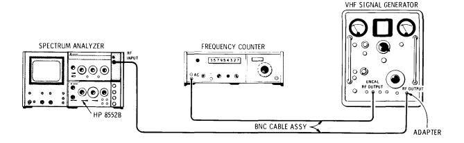
Figure 4-5. 10 kHz Bandwidth Accuracy Test Setup
