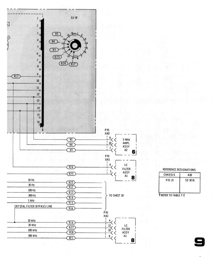
Figure 8-30. Amplifier/Filter Control Circuits
