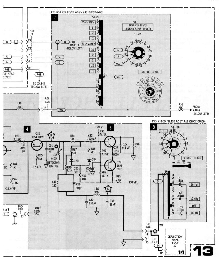
Figure 8-39. Log/Linear Amplifier (2 of 2)
