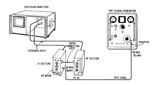
Figure 5-15. 44 MHz Rejection Adjustment Test Setup
