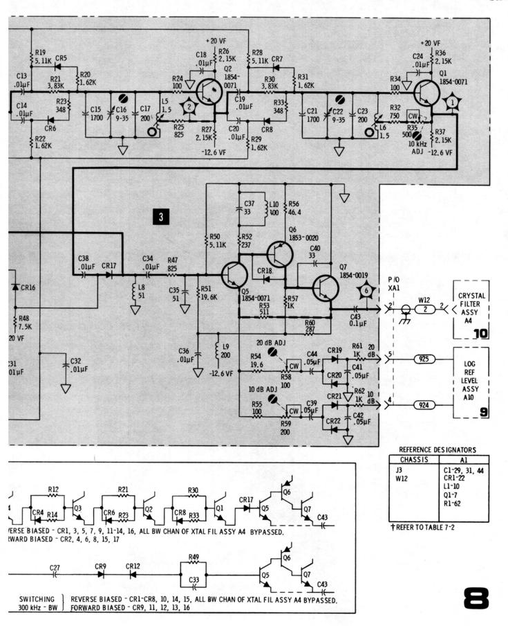
Figure 8-29. LC Bandwidth Filter
