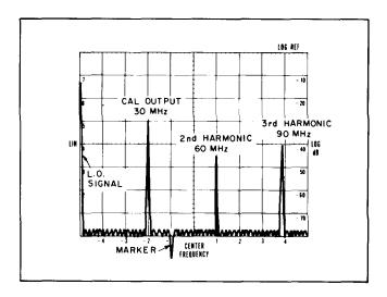
Figure 4-1. 30 MHz Calibrator Signal & Harmonics
