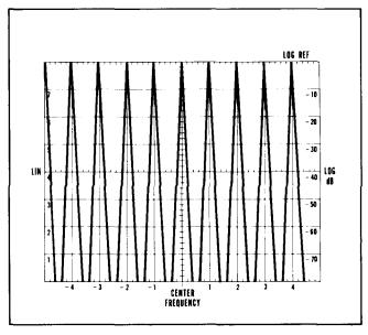
Figure 5-14. 50 MHz Bandpass Flatness Display
