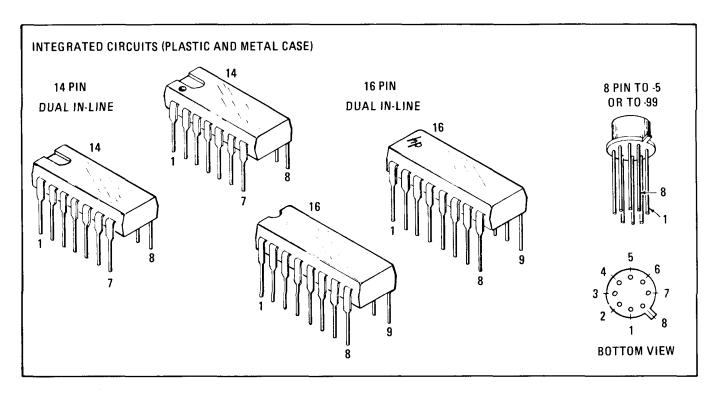
Figure 8-4. Integrated Circuit Packaging
