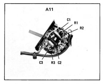
Figure 8-11. Video Filter Assembly A11
