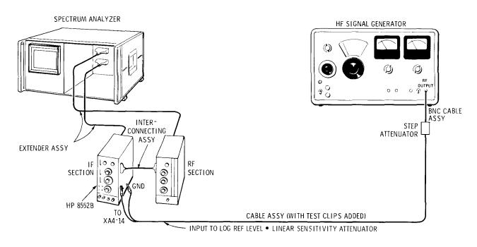
Figure 5-5. Vertical Deflection Amplifier Test Setup
