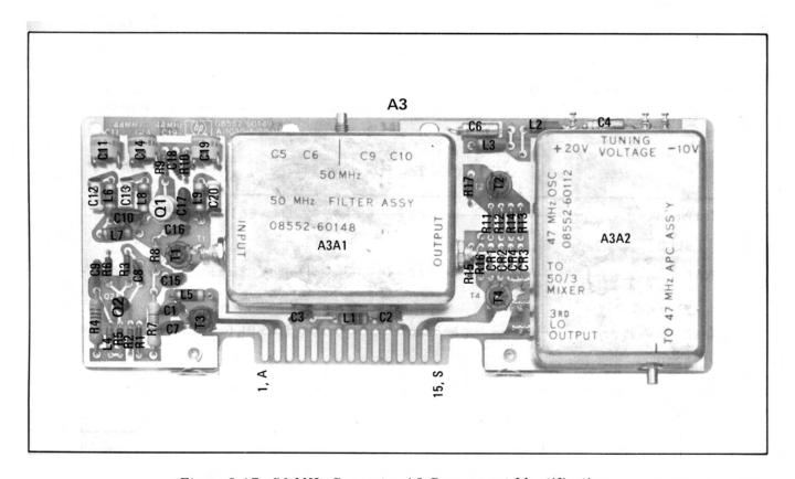
Figure 8-17. 50 MHz Converter A3 Component Identification
