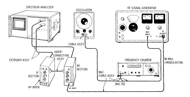
Figure 5-4. Final Scan Time Adjustment Test Setup
