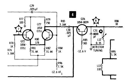
Figure 7-5. Log/Linear Amplifier Partial Schematic (Part of Change J)
