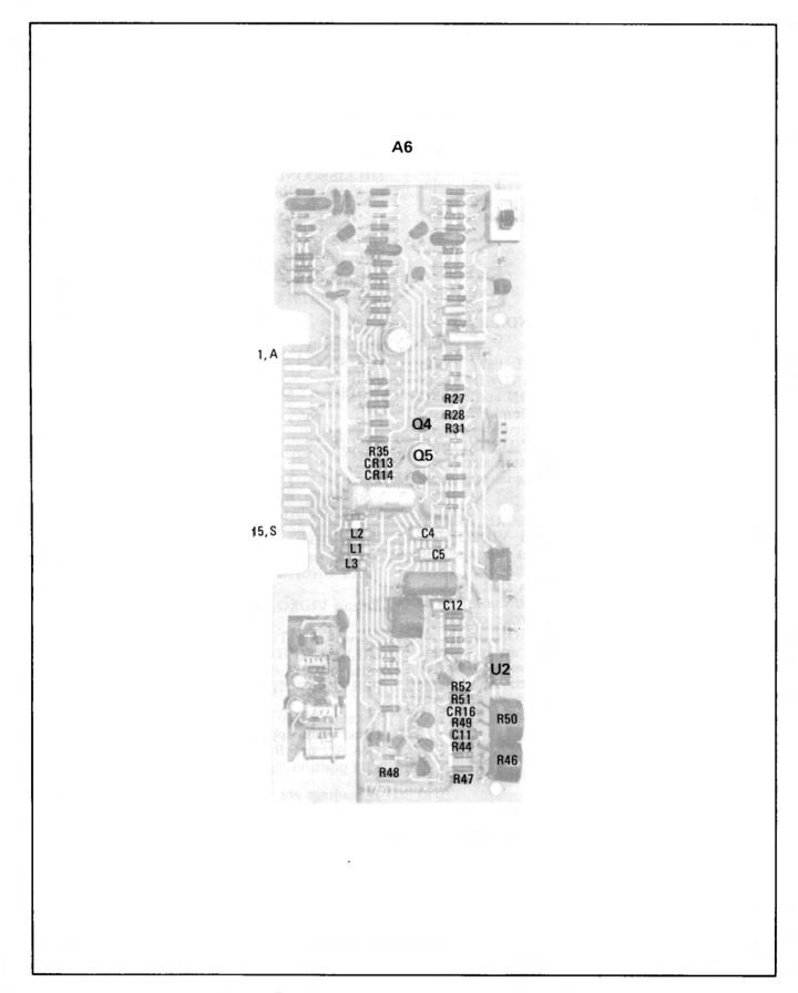
Figure 8-44. P/O Scan Generator A6 Component Identification
