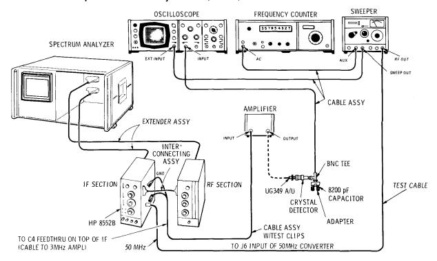
Figure 5-12. 50 MHz IF Bandpass Adjustment Test Setup
