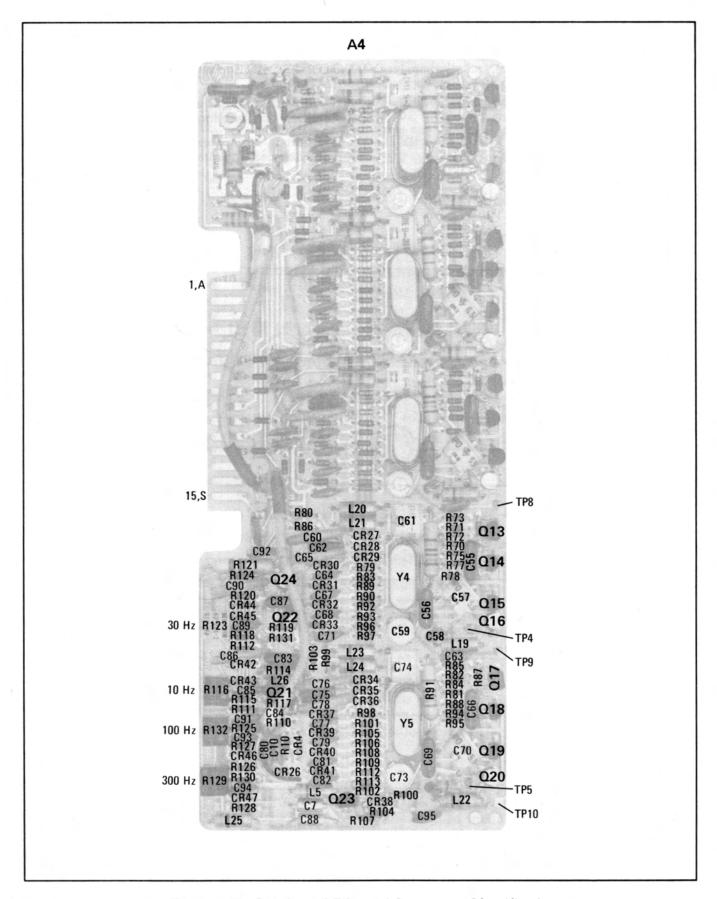
Figure 8-33. P/O Crystal Filter A4 Component Identification
