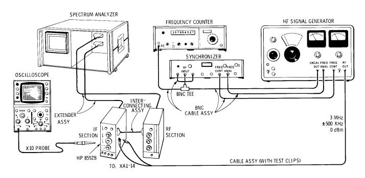
Figure 5-7. Crystal Filter Fine Adjustment Test Setup
