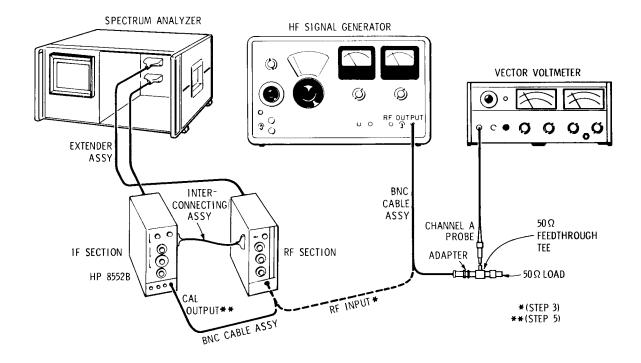
Figure 5-16. 30 MHz Calibration Amplitude Adjustment Setup
