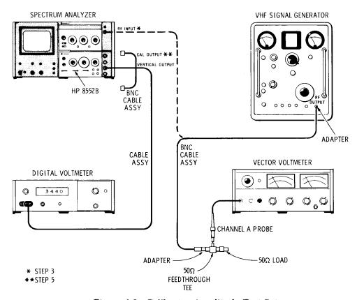
Figure 4-3. Calibrator Amplitude Test Setup
