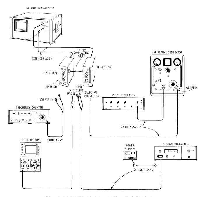
Figure 5-10. 47 MHz LO Automatic Phase Lock Test Setup
