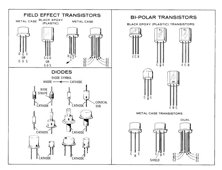
Figure 8-3. Examples of Diode and Transistor Marking Methods
