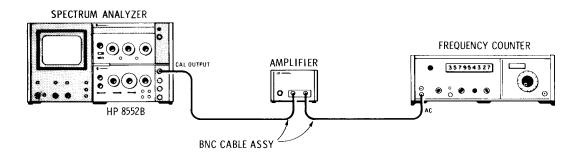
Figure 4-4. Calibrator Frequency Check Test Setup
