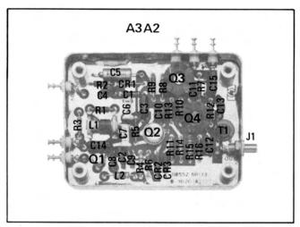
Figure 8-16. 47 MHz LO A3A2 Component Identification
