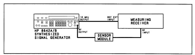
Figure 4-2. Harmonics Test Setup
