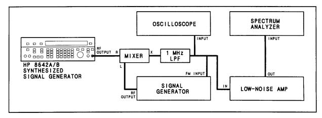
Figure 4–12. SSB Phase Noise Test Setup (Optional)
