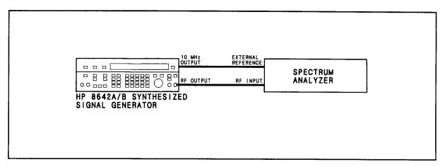
Figure 4-9. Harmonics and Spurious Test Setup
