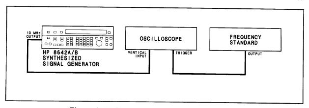
Figure 4-15. Internal Time Base Aging Rate Test Setup
