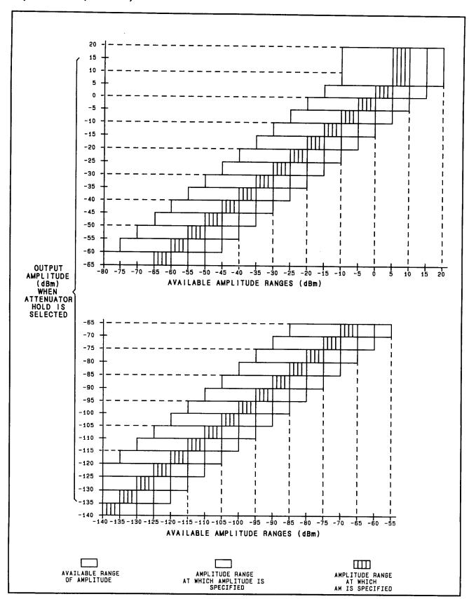
Figure 3-9. Attenuator Range Hold; Amplitude and AM Ranges
