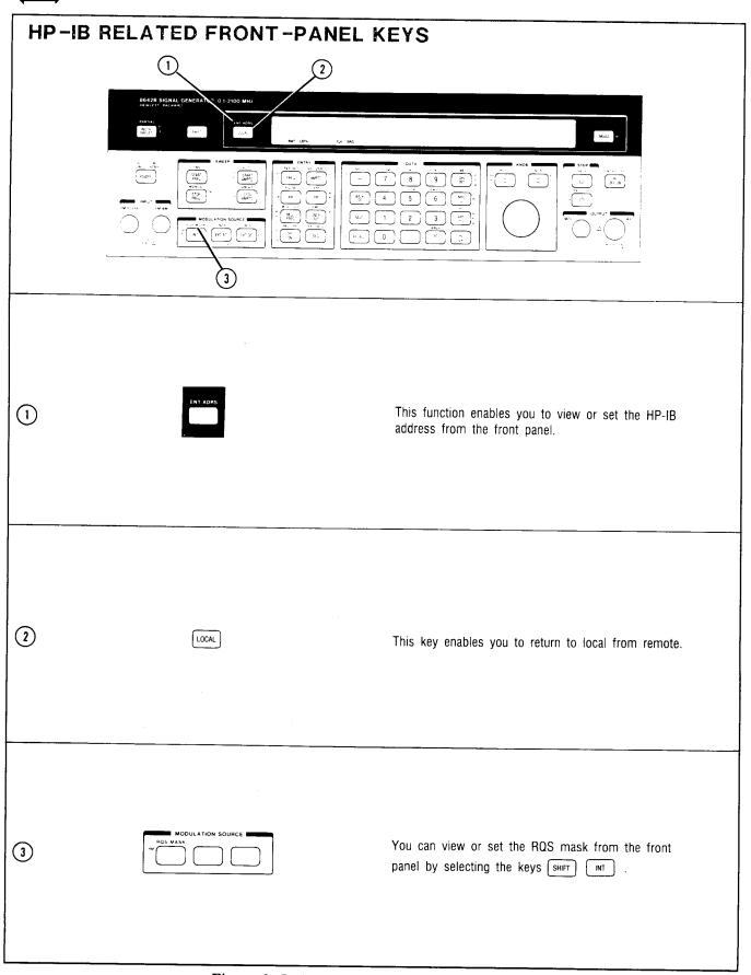
Figure 3-5. HP-IB Related Front-Panel Keys
