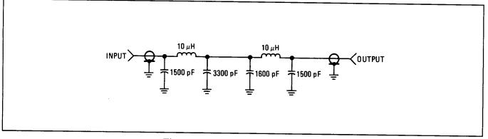
Figure 1-1. 1 MHz Low-Pass Filter
