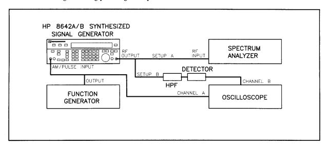
Figure 4-13. Pulse Test Setup
