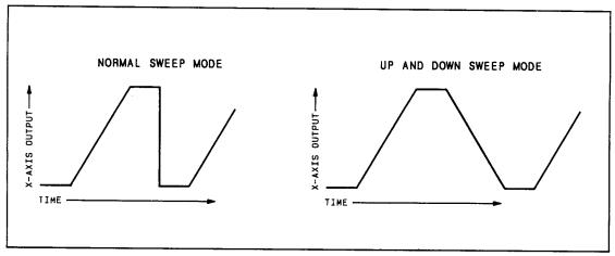
Figure 3-7. Sweep Waveforms
