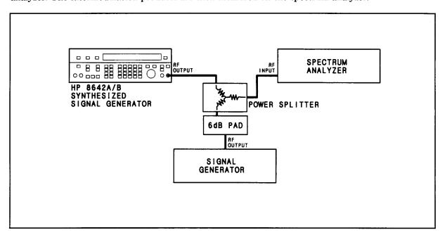
Figure 4-10. Intermodulation Test Setup
