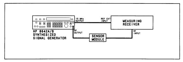
Figure 4-4. Residuals Test Setup
