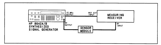
Figure 4-1. Level Accuracy and Flatness Test Setup
