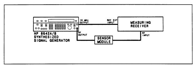
Figure 4-5. AM, FM, and PM Test Setup
