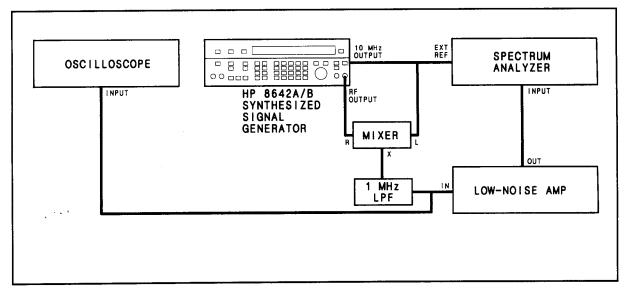
Figure 4-11. SSB Phase Noise Test Setup
