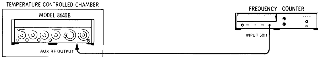
Figure 4-2. Frequency stability vs Temperature Test Setup
