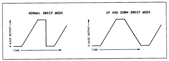
Figure 3-10. Sweep Waveforms
