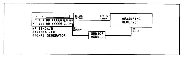
Figure 4-3. Pulse Test Setup
