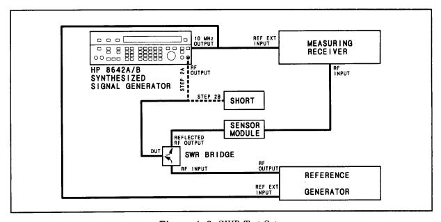
Figure 4-8. SWR Test Setup
