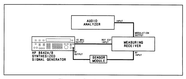
Figure 4-6. FM Distortion Test Setup
