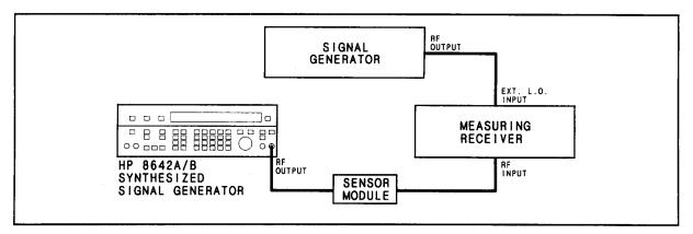
Figure 4-14. Residual Test Setup
