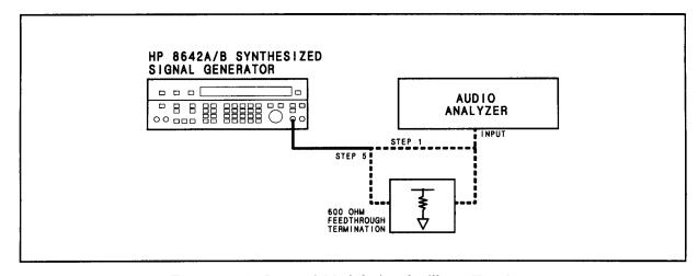
Figure 4-7. Internal Modulation Oscillator Test Setup
