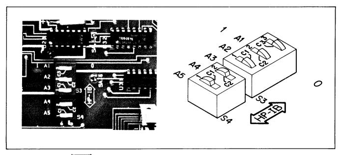
HP-IB Figure 2-4. HP-IB Address Switch Location and Settings
