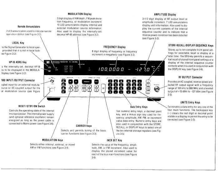
Figure 3-1. Simplified Front Panel Features
