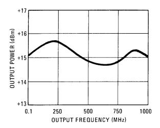
Typical maximum power output versus frequency (output set to +17 dBm).
