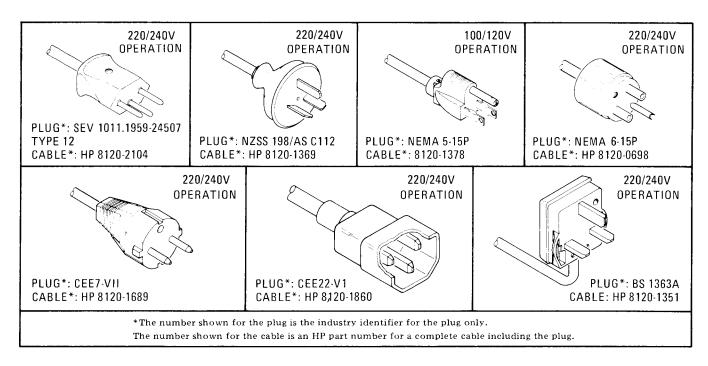
Figure 2-2. Power Cable and Mains Plug Part Numbers
