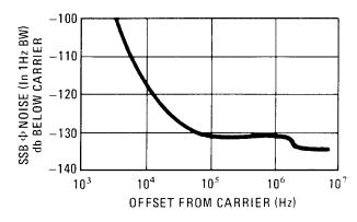
Typical SSB  $\phi$  Noise,  $f_c = 450$  MHz.
