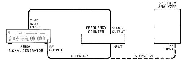
Figure 3-8. Test Setup for Basic Functional Checks
