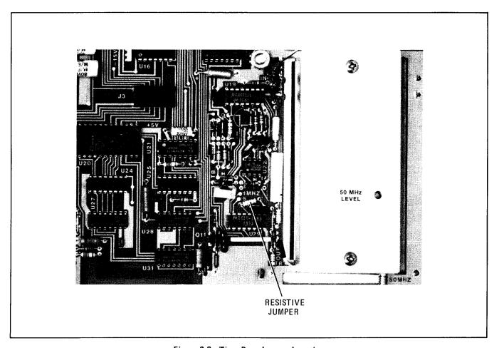
Figure 2-3. Time Base Jumper Location
