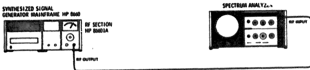
Figure 4-5. Harmonic Signal Test Setup
