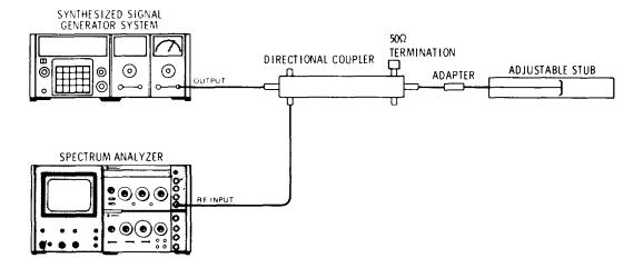
Figure 4-7. Output Impedance Test Setup
