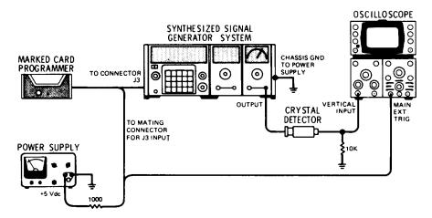
Figure 4-3. Output Level Switching Time Test Setup
