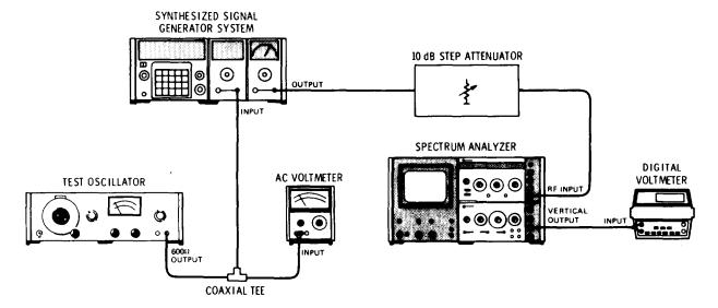
Figure 5-3. Amplitude Modulation Input Circuit Adjustment Test Setup
