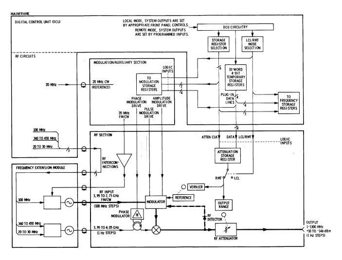
Figure 8-6. System Troubleshooting Block Diagram
