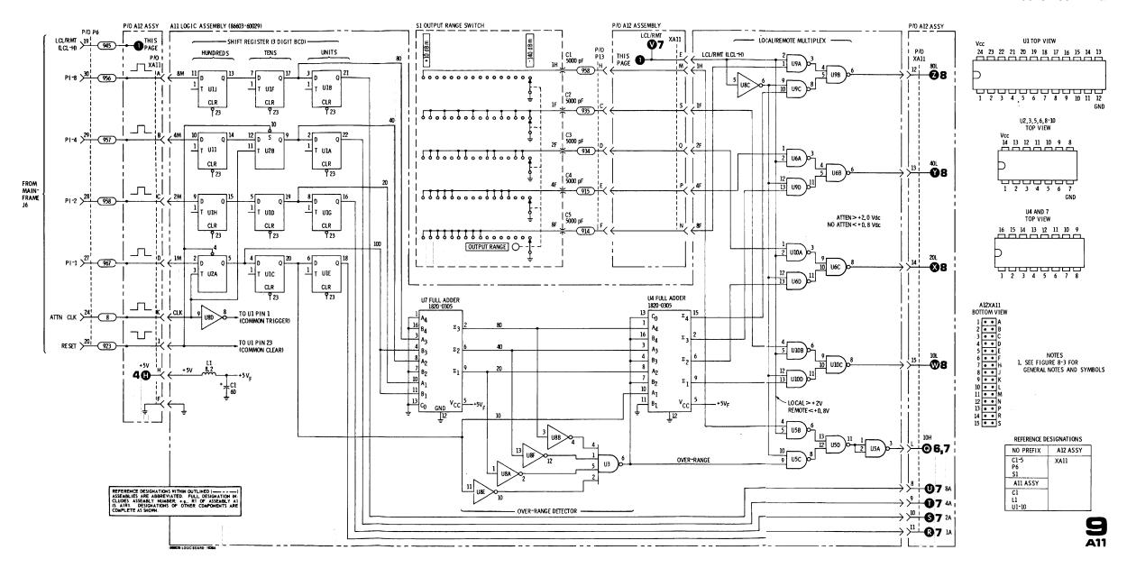
Figure 8-24. A11 Logic Assembly Schematic Diagram.
