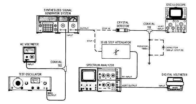
Figure 4-6. Amplitude Modulation Depth and 3 dB Bandwidth Test Setup
