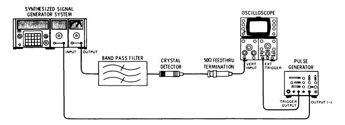
Figure 4-5. Pulse Modulation Risetime Test Setup
