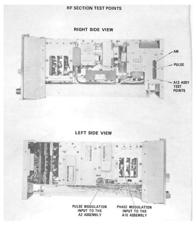
Figure 8-4. System Test Point Locations
