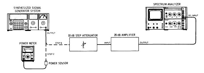
Figure 4-4B. Output Accuracy Test Setup (Alternate Procedure)
