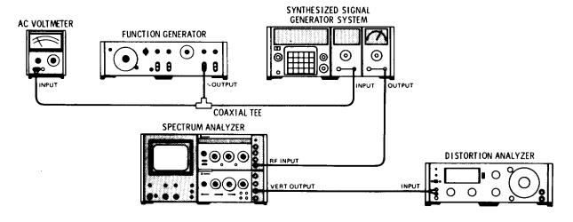
Figure 4-11. Amplitude Modulation Distortion Test Setup.
