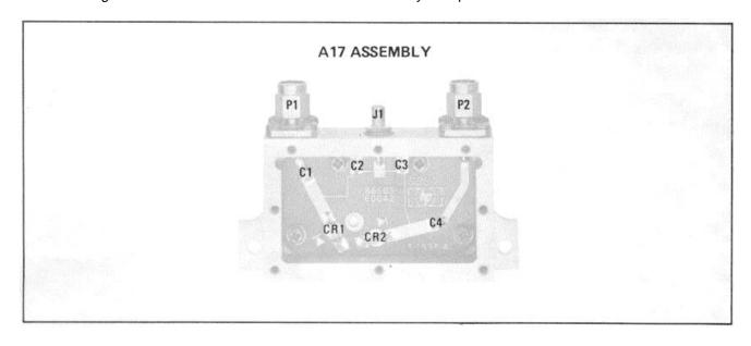
Figure 8-13. A17 Phase Modulator Assembly component Locations
