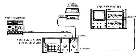
Figure 5-4. Phase Modulator Driver Frequency Response Adjustment Test Setup
