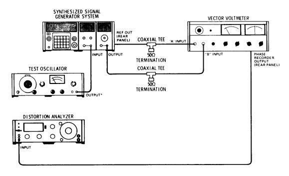
Figure 4-17A. Phase Modulation Distortion Test Setup
