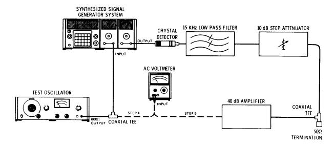
Figure 4-9. Signal-to-AM Noise Test Setup
