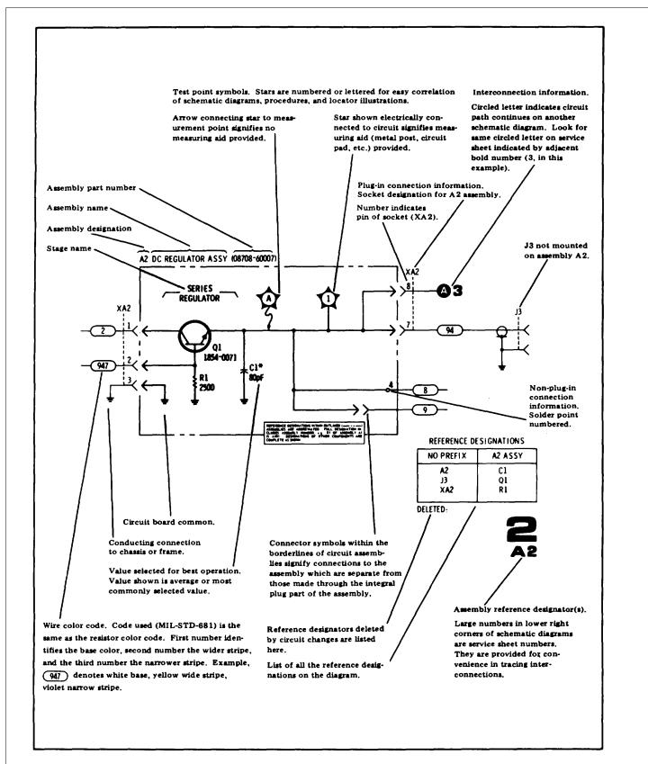
Figure 8-3. Schematic Diagram Notes (3 of 3)
