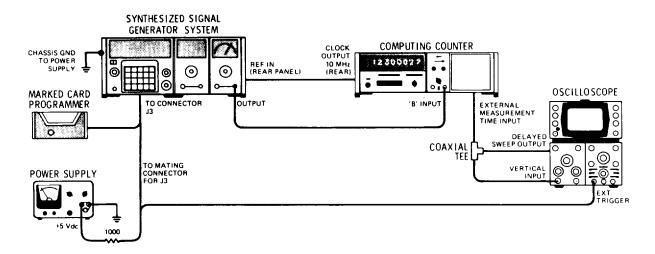
Figure 4-2. Frequency Switching Time Test Setup
