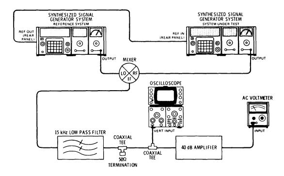
Figure 4-8. Signal-to-Phase Nose Ratio Test Setup
