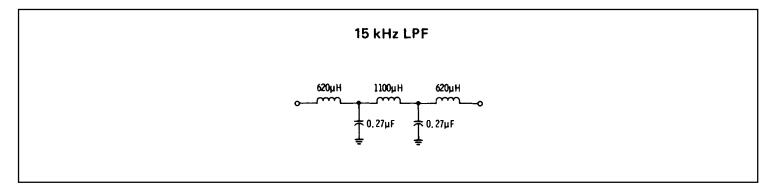
Figure 1-3. 15 kHz Low Pass Filter
