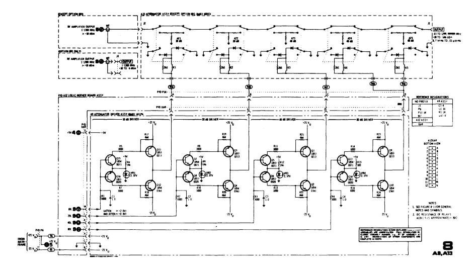
Figure 8-22. Attenuator Section Schematic Diagram (P/O Change 1)
