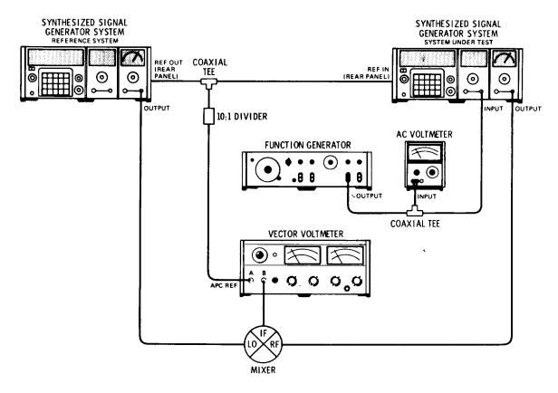
Figure 4-12. Incidental Phase Modulation Test Setup
