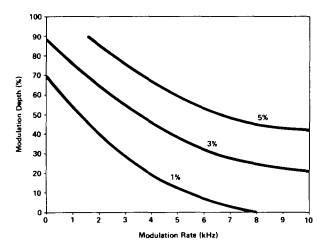
Typical AM Distortion (Center Frequency <10 MHz)
