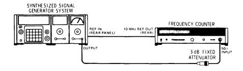
Figure 4-1. Frequency Range Test Setup
