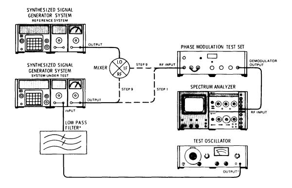
Figure 4-17B. Phase Modulation Distortion Test Setup (Alternate Procedure)
