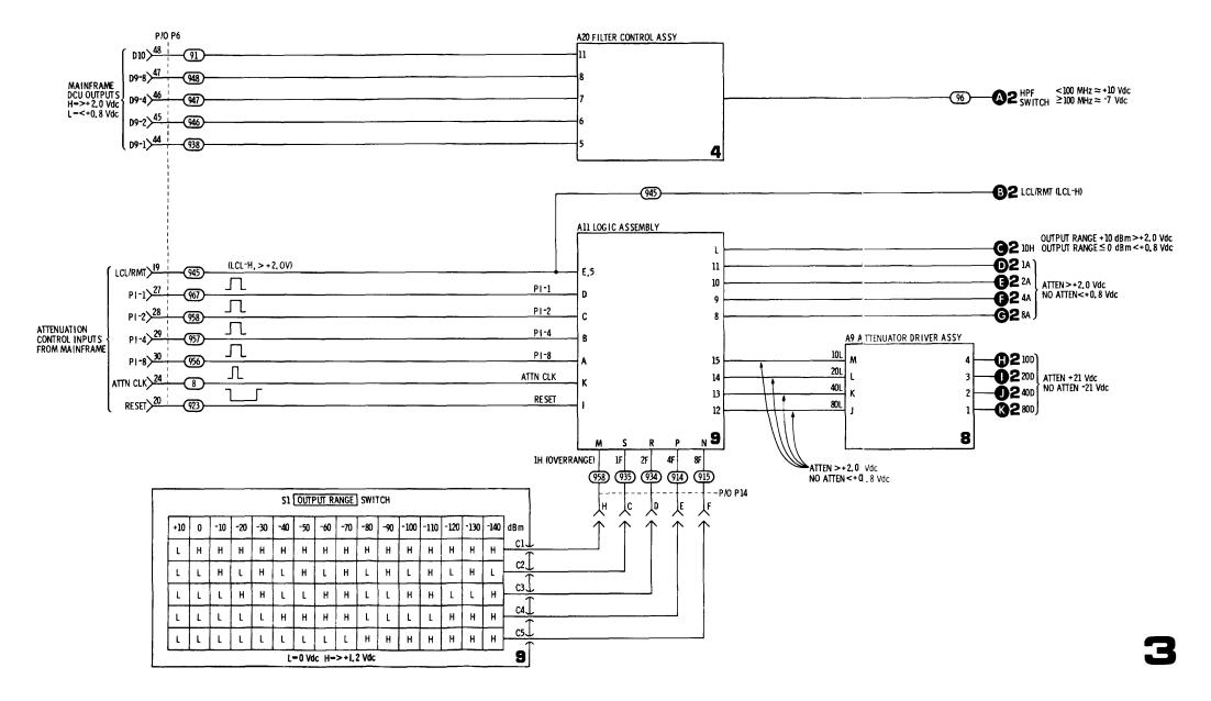
Figure 8-9. Logic Troubleshooting Block Diagram
