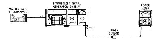
Figure 5-2. 1 dB Step Attenuator Adjustment Test Setup
