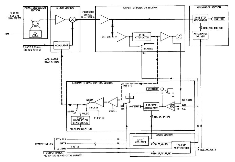
Figure 8-7. RF Section Simplified Block Diagram
