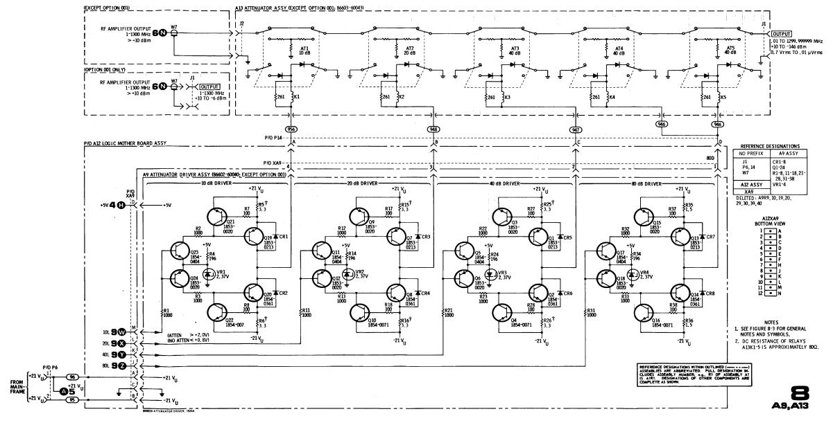
Figure 8-22. Attenuator Section Schematic Diagram
