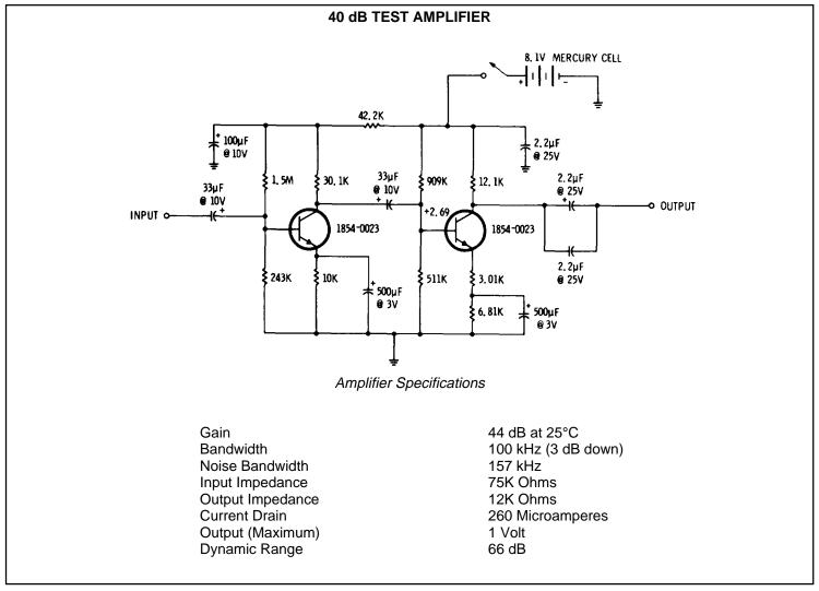
Figure 1-2. 40 dB Test Amlifier
