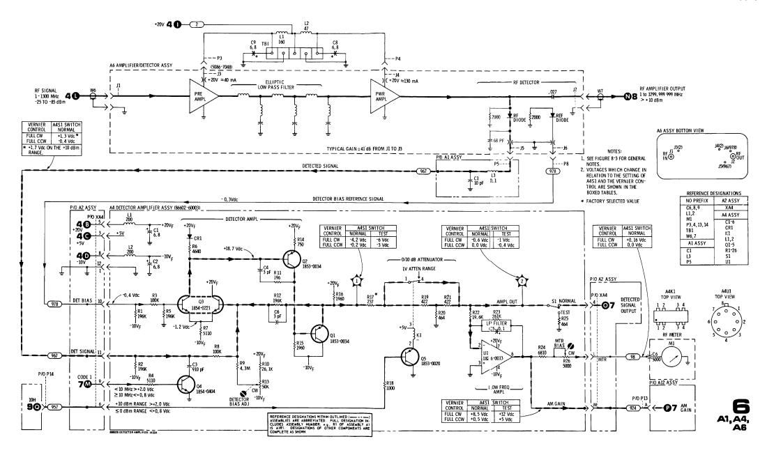
Figure 8-16. Amplifier/Detector Section Schematic Diagram
