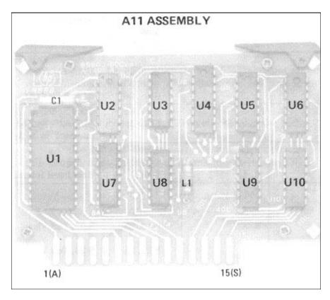
Figure 8-23. A11 Logic Assembly Component Locations.
