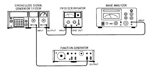
Figure 4-13. Frequency Modulation Distortion Test Setup
