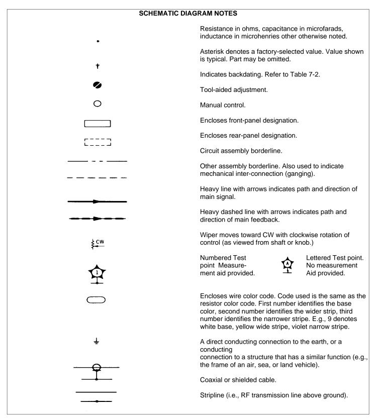
Figure 8-3. Schematic Diagram Notes (1 of 3)
