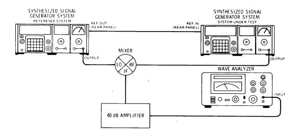
Figure 4-15. Narrowband Spurious Signal Test Setup.
