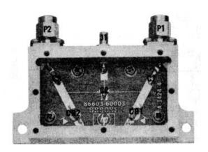
Figure 7-4. A17 Phase Modulator Assembly Component Locations (Change C)
