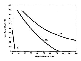
Typical AM Distortion (Center Frequency > 10 MHz)
