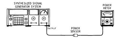
Figure 5-1. RF Output Level Adjustment Test Setup
