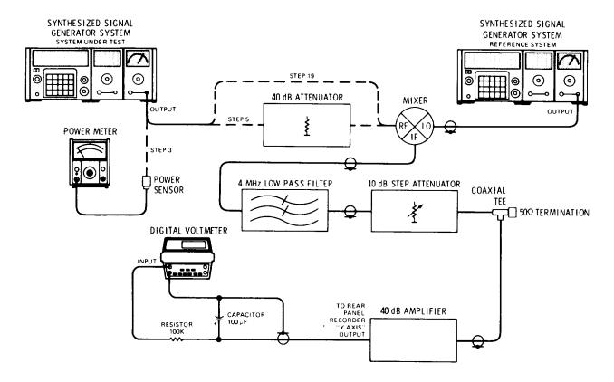
Figure 4-4A. Output Accuracy Test Setup
