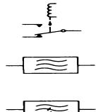
Arrows on relays indicate direction of arm movement when energized.
