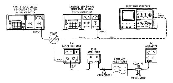
Figure 4-10. Residual FM Test Setup
