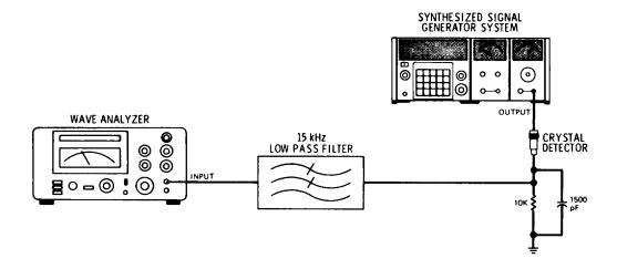
Figure 4-14. Incidental AM Test Setup
