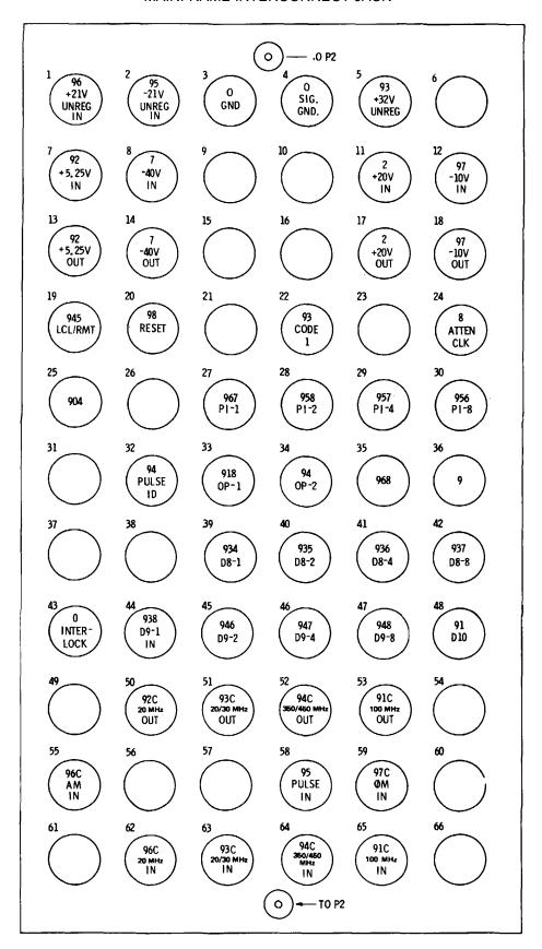
Figure 8-5. Mainframe Interconnect Jack
