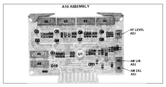
Figure 8-18. A10 Reference Assembly Component Locations
