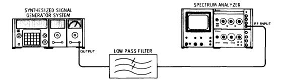
Figure 4-16. Wideband Spurious Signal Test Setup
