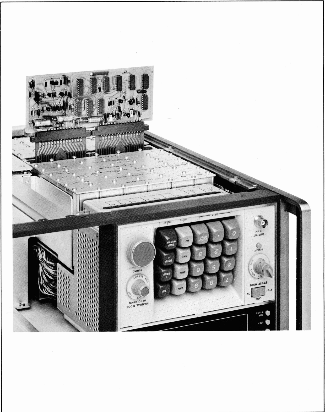
Figure 8-4. Model 8660B With Circuit Board Extended for Maintenance
