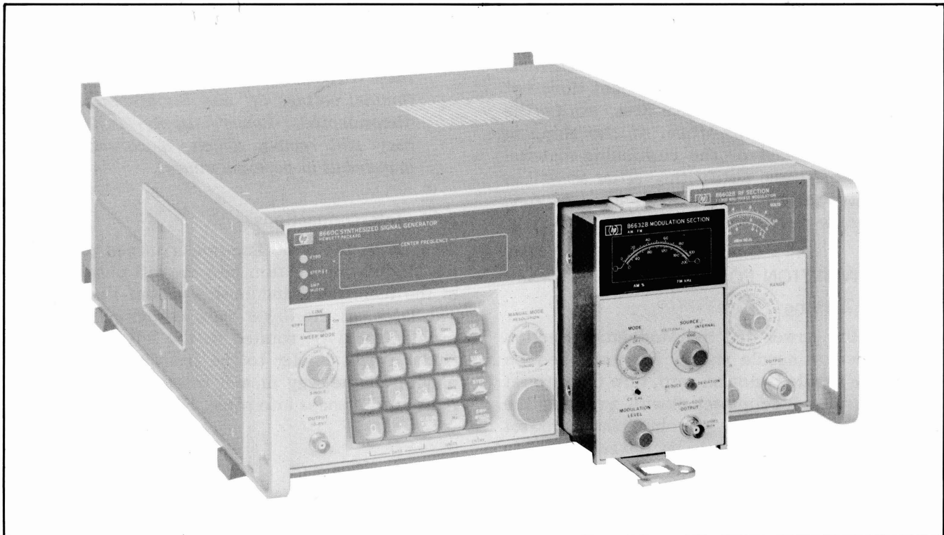
Figure 2-1. Model 86632B Being Installed in Mainframe
