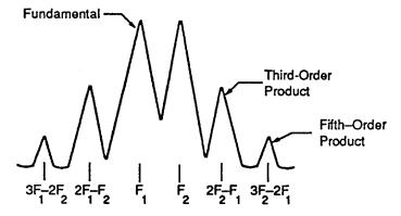
located close to the original signals at 2F2 - F1 and 2F1 - F2, span should be reduced to as narrow as possible while still allowing the distortion products to be displayed.
