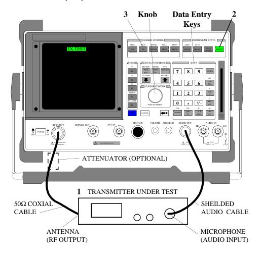
1. Connect the Transmitter as shown.
