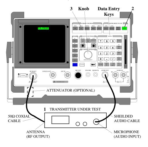
1. Connect the Transmitter as shown.
