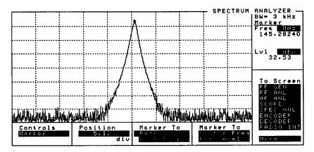
Relative frequency and amplitude measurements such as filter bandwidth, duplexer rejection/insertion loss, or harmonic level can be performed using the "Delta" marker function.
