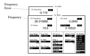
Frequency or frequency error is displayed as shown.
