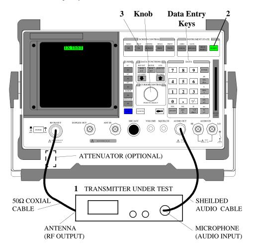
1. Connect the Transmitter as shown.
