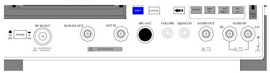
RF IN/OUT Connector – type-N female connector for output signals from the RF Generator, and input signals (60 Watts continuous, or 100 Watts for 10 sec/min) to the RF Analyzer. Nominal impedance is  $50\Omega$ .
