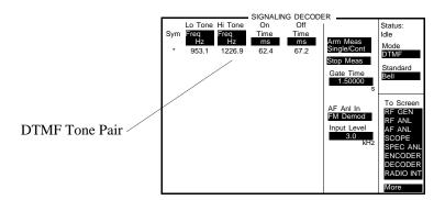
To Measure deviation of the DTMF on the Test Set:
