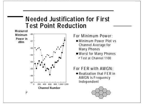
The database can provide justification for the reduction of test points. For the minimum power test, the average of many phones is plotted as a function of frequency. Also shown is the worst case measurement of many phones. It may be interesting to plot a 3 or 4 sigma line from the average, as well.
