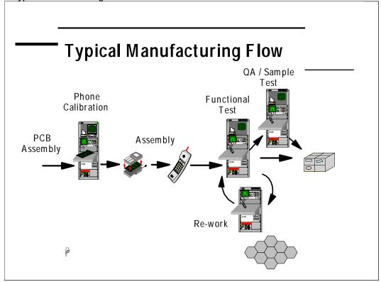
A typical production line is depicted here. Not shown is the surface mount printed circuit board assembly step. The loaded boards are usually tested in board form. Often this is in fixtures that behave much like the phone housing and enclosures. Calibration is done in this state.
