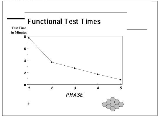
The test times for functional test have been reduced by a factor of almost 10! The initial test list was very detailed, while the final test list was very focused. Substantial improvements were made by using the concurrent measurement capability of the HP 8924C.
