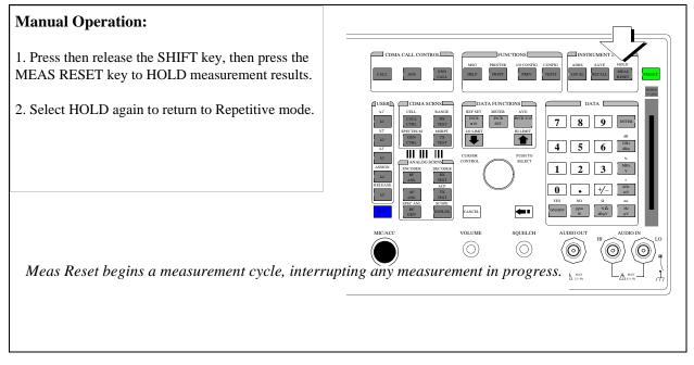
Triggering Analog Measurements In Local Mode (Front Panel Operation)
