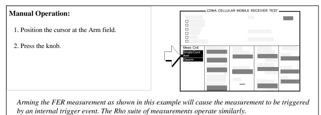
Selecting the Disarm field will stop the currently executing measurement cycle for the FER or Rho Suite of Measurements.
