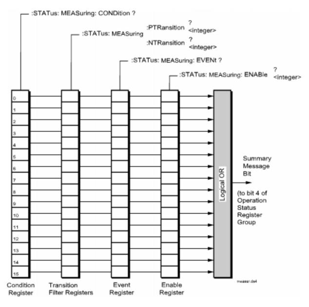
Figure 22 Measuring Status Register Group
