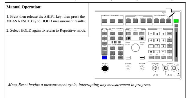
Triggering CDMA Measurements In Local Mode (Front Panel Operation)
