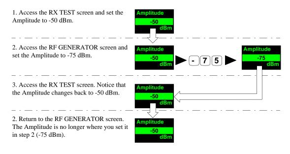
Since the RX TEST screen has priority control over this field, the RF GENERATOR screen's Amplitude setting changed when RX TEST was accessed.
