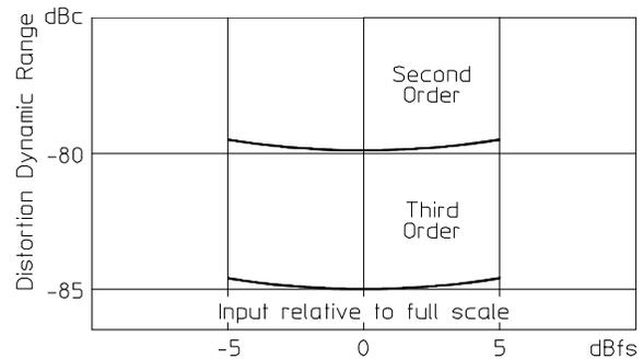
**Typical harmonic and intermodulation distortion**
