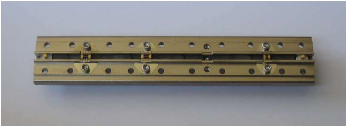
Pad carrier. Third pad is missing. The fourth pad is 10 dB. It is shorter. The SMA connectors are at both ends.
