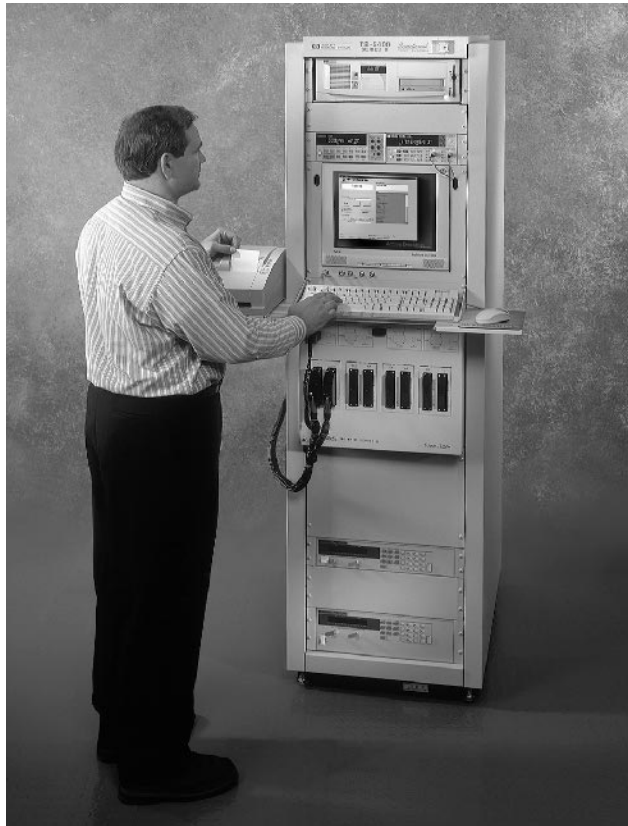
The TS-5400 Series II Automotive Electronics Functional Test Platform. Shown is the E8785A family member with the optional express connect interface connector assembly (ICA).
