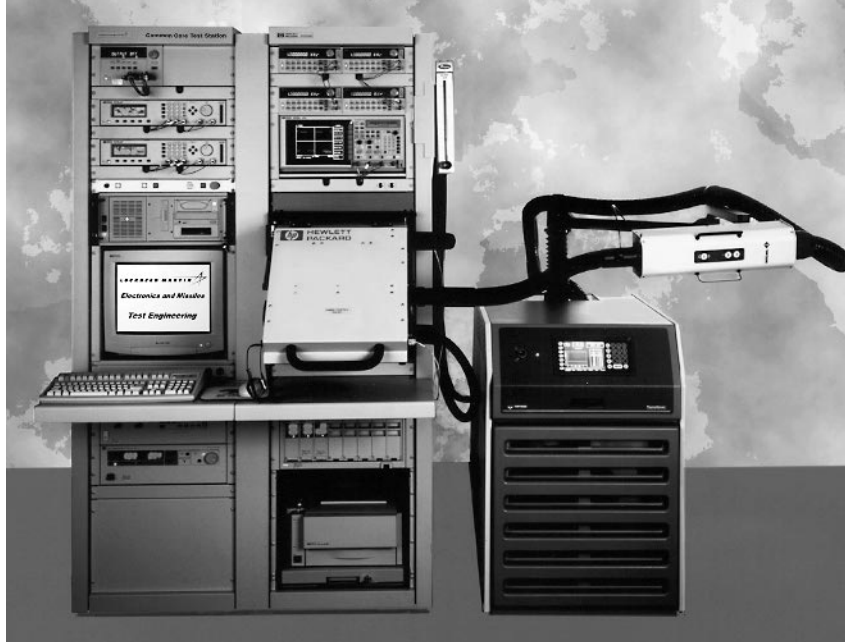
Hellfire II Common Core Test Station with Temperature Forcing Unit.
