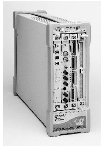
The HP E8408A is HP's smallest footprint, lowest-priced C-size mainframe.
