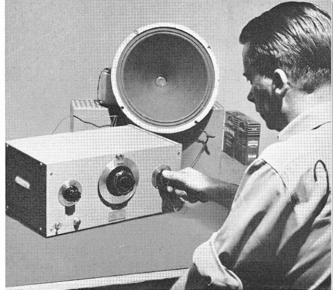
This Model 200B oscillator is being used to check the resonate frequency of a speaker.
