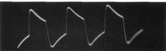
Square Wave Distortion from poor response at both low and high frequency. (A typical amplifier oscillogram.)
