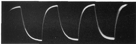
Square Wave Distortion from poor high frequency response.
