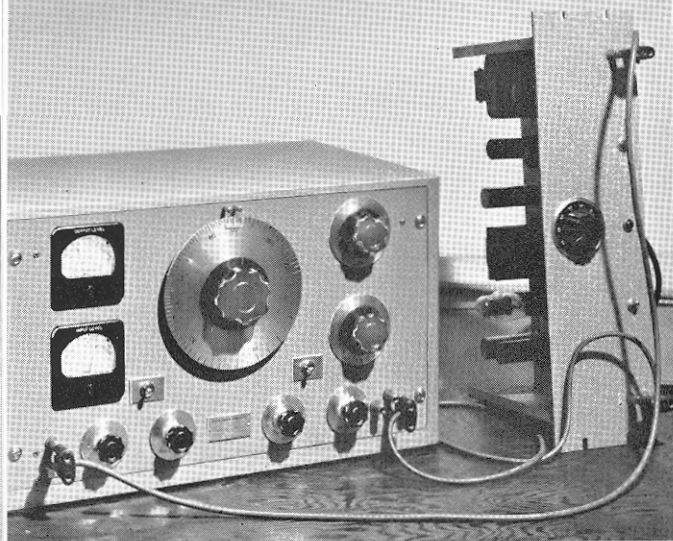
A Model 205AG is connected to measure the gain of an amplifier.
