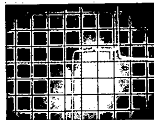
System Profile: Reflection pattern as seen by looking down a transmission system. The pattern reveals a low impedance cable (off screen) connected to a 69\Omega cable. 27 ft from the connector is an inductive defect; 20 ft farther along is a capacitive defect from a pinched cable; 8 ft from the pinch is a 67\Omega termination.
