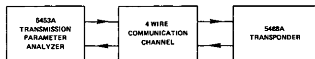
Figure 1. Typical point-to-point measurement. The 5468A is controlled by the 5453A over the channel to be tested.
