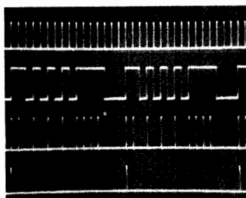
External clock NRZ Output (16 bit continuous word recycling) RZ Output signal First bit synch pulse
