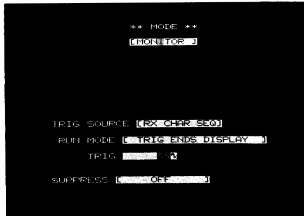
Most network problems can be isolated using the Monitor mode. Parameters for the Monitor menu set the trigger type, manner of data collection, trigger, and specify characters to be suppressed.
