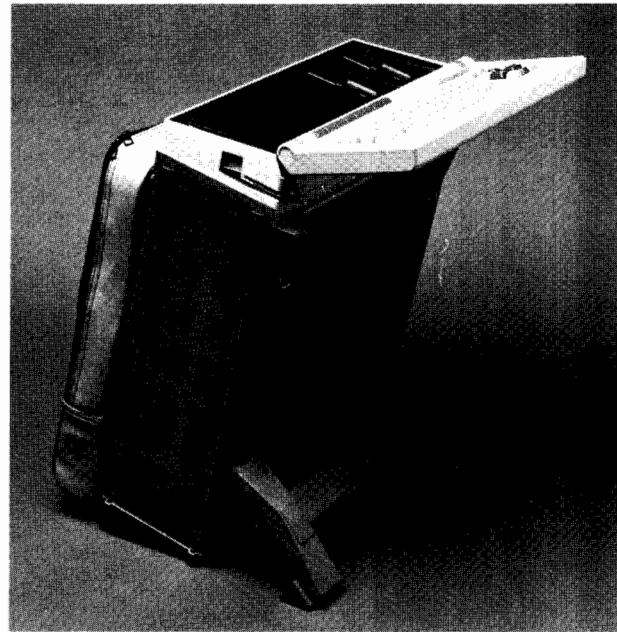
Figure 2. Model 64110A Development Station, with integral, dual flexible disc drives, has a hinged keyboard and adjustable legs, for easy use in a wide variety of environments.
