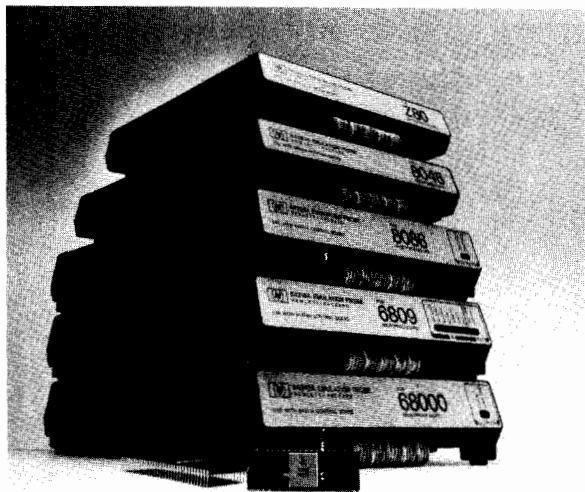
Figure 4. Emulation subsystems are available for a variety of 8-bit and 16-bit microprocessors. Emulation pods are shown for some of the supported processors.
