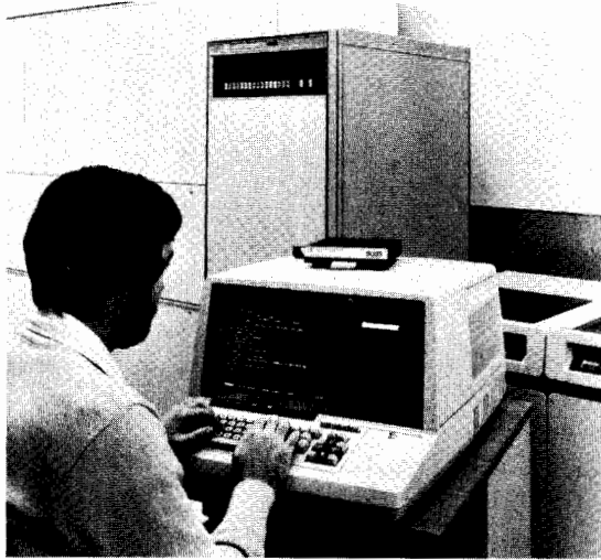
Figure 10. By combining a hardware analyzer and software analyzer via the Intermodule Bus (IMB), one analyzer can trigger or arm the second analyzer for interactive measurements.
