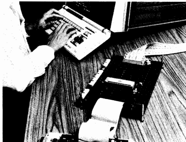
A user-definable emulator provides emulation support for microprocessors for which there are no processor-specific 64000 System emulators available.
