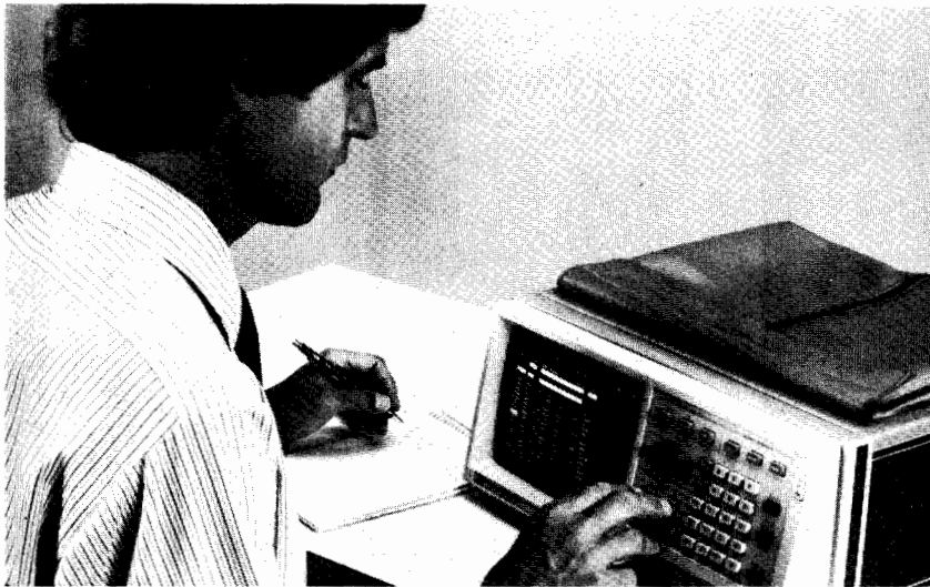
Benchtop logic analyzers provide state, timing and performance analysis for troubleshooting and optimizing digital systems in the laboratory and at remote sites.
