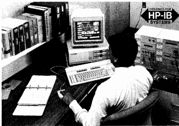
The HP Touchscreen II PC, with a Winchester disc drive, is ideal for use with test and measurement instruments.
