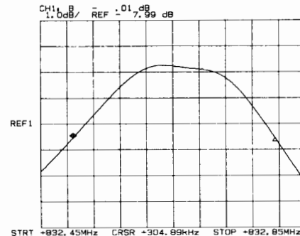
HP 8341B 400 kHz sweep of 832 MHz SAW resonator
