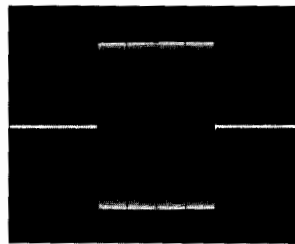
HP 8340B/8349B/83554A Pulse Performance at 35 GHz. Pulse width = 5 \mu s.
