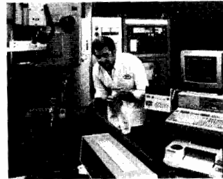
Machine tool calibration with the HP 5528A
