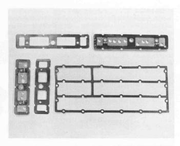
Fig. 3. Copper waffled gaskets seal the interfaces between the extrusions and the extrusion covers and motherboards.
