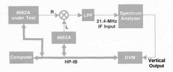
**Fig. 14.** System to measure the spurious output of the 8662A uses a 21.4-MHz spectrum analyzer IF section and a second 8662A as a swept local oscillator. The second 8662Aimproves the analyzer's phase noise.
