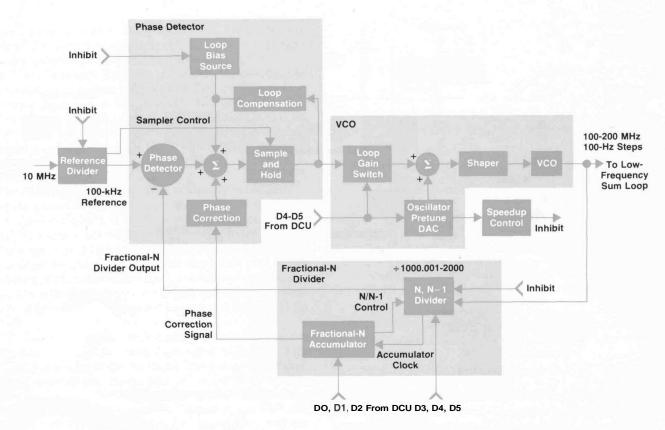
Fig. 10. Fractional-N loop provides the lower six decades of frequency resolution. Its output has a frequency of 100.0001 to 200 MHz in 100-Hz steps. This is divided by 1000 to give 0.1-Hasteps at the 8662A output.
