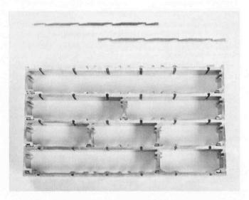
Fig. 1. Interlocking extrusions provide a low-cost modular approach to internal shielding in the 8662A Synthesized Signal Generator.
