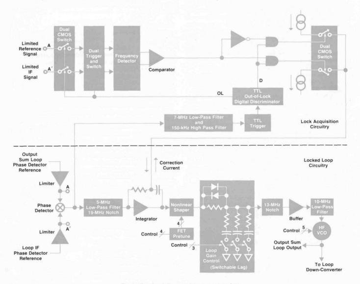
Fig. 6. Functional diagram of the output sum loop.
