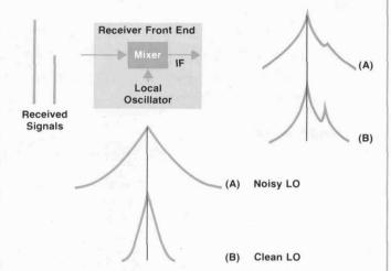
**Fig. 1.** Sideband noise on the local oscillator output limits the resolving power of heterodyne receivers.
