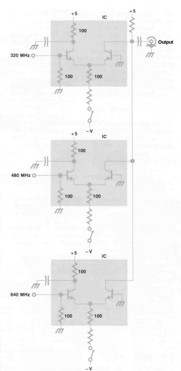
Fig. 3. The higher frequencies in the reference section are switched by a form of ECL multiplexer using several monolithic differential pairs connected to a common collector resistor.
