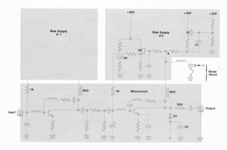
Fig. 3. 8662A output amplifier is a two-stage feedback amplifier realized as a thin-film microcircuit on a sapphire substrate. It provides 17 dB gain from 10 kHz to 1280MHz.
