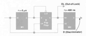
Fig. 7. The out-of-lock digital discriminator generates the out-of-lock signal (OL) that controls several functions in the output sum loop. It also produces a signal (D) that represents the difference between the loop input and output frequencies.
