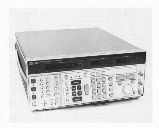
Fig. 1. Exceptionally low phase noise and spurious output make Model 8662A Synthesized Signal Generator suitable for such demanding applications as receiver adjacent channel selectivity measurements with closely spaced channels and low-noise local oscillator service. Fast frequency switching and sweep capability make the 8662A useful in frequency-agile and swept local oscillato applications. All functions are remotely programmable.
