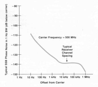
Fig. 3. Typical 8662A phase noise performance.
