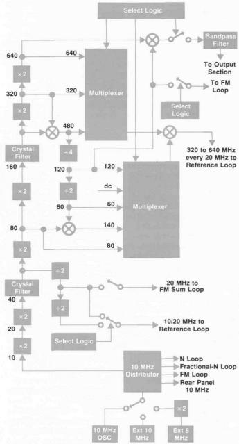
Fig. 2. 8662A reference section derives various frequencies by multiplying, dividing, and mixing the output of the internal crystal reference oscillator or an external standard.
