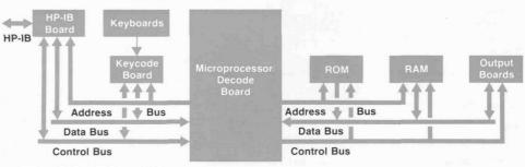
Fig. 1. Digital control unit of the 8662A Synthesized Signal Generator exercises 132 control lines.
