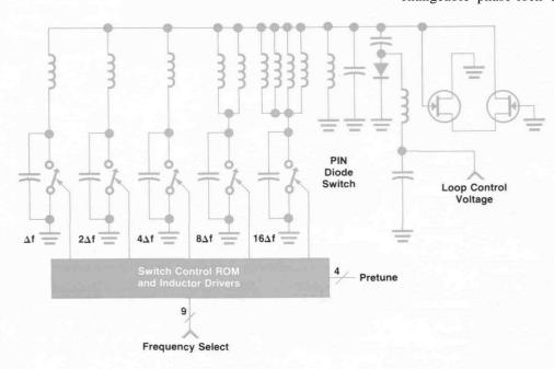
Fig. 5. The VCO in the output sum loop is this 320-to-640-MHz switched reactance oscillator. It meets requirements of low phase noise and low tuning sensitivity.
