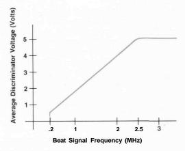
Fig. 8. Average value of the digital discriminator'sD output is a function of the beat or difference frequency between the input and output of the output sum loop. This signal provides the magnitude of the feedback to steer the loop into lock.
