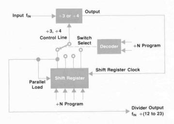
**Fig. 11.** This 12-to-23 integer divider is used in the phase-locked loop that generates 122 to 221 MHz in 1-MHzsteps. A separate circuit controls a fractional digit to give divide numbers of 12.2 to 22.1.
