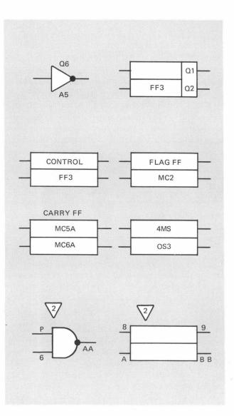
3-6. On logic diagrams which correlate to a schematic diagram of the same circuit, the active components of the element may also be designated, as shown at left. This is primarily an aid in troubleshooting. The symbol shown for the switching element is a variation of the standard symbol for this special prupose.
