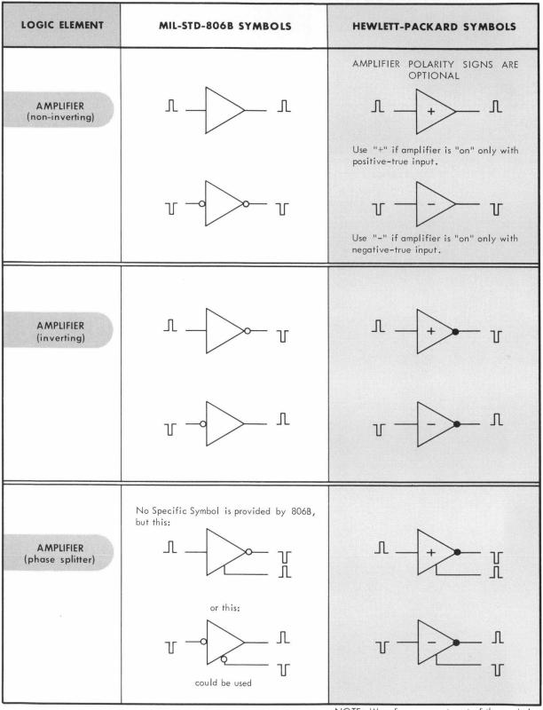
NOTE: Waveforms are not part of the symbols; they are shown to illustrate the logic
